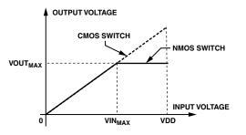
Figure 6. Transfer Function of a NMOS Switch
