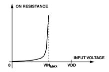
Figure 5. On Resistance Profile of a NMOS Switch
