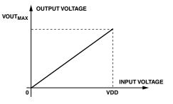
Figure 3. Transfer Function of a CMOS Switch
