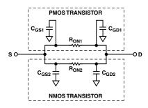
Figure 4. Small Signal Equivalent Circuit
