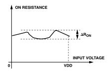
Figure 2. On Resistance Profile of a CMOS Switch
