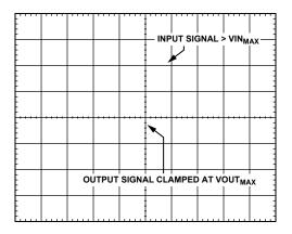
Figure 7. Output Signal Clamping Effect
