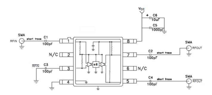
Figure 3 – Application Circuit
