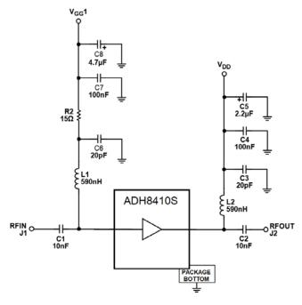
Figure 3 - Typical application Circuit
