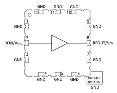
Figure 1 – Functional Block Diagram 1/ 1/ Package top view
