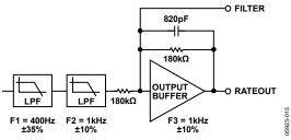
Figure 14. Simplified Filtering Network
