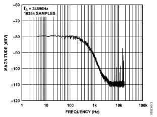
Figure 12. Noise Density vs. Frequency
