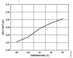
Figure 8. Self-Test vs. Temperature, VCC = 5 V
