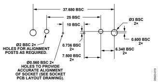
Figure 18. Interface Board Hole Locations for Bulkhead Mount
