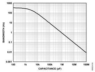
Figure 15. Bandwidth vs. Capacitance
