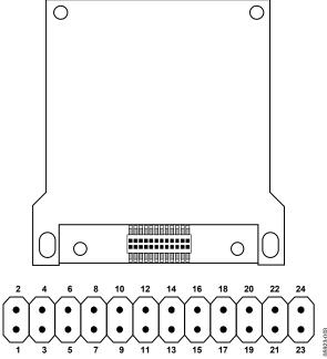
Figure 3. Pin Configuration (Connector-Up View)
