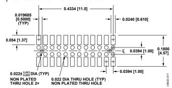
Figure 16. Mating Socket Recommended Pad Layout Dimensions are shown in inches (millimeters)
