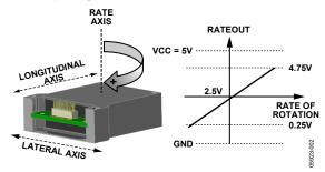
Figure 2. Rotational Measurement Orientation
