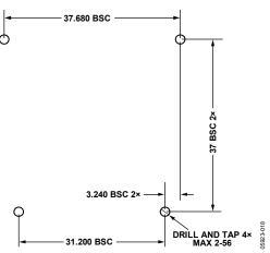
Figure 17. Bulkhead Mount Attachment Hole Locations
