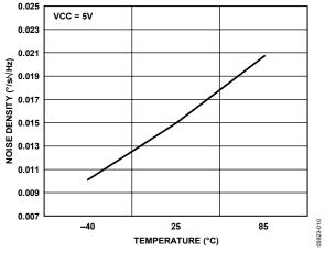
Figure 10. Noise Density vs. Temperature, VCC = 5 V
