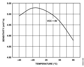
Figure 6. Gain Sensitivity vs. Temperature @ ±300°/sec
