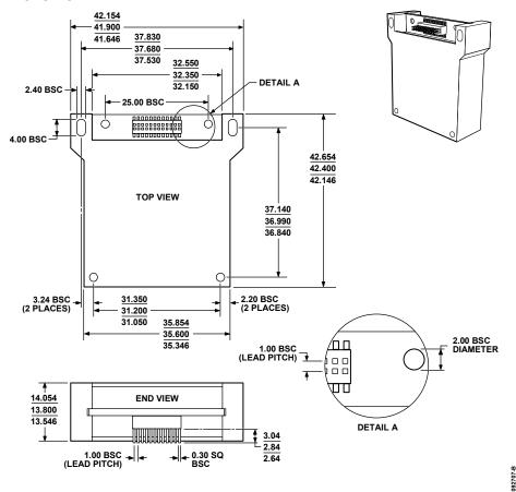
Figure 20. ADIS16120 PCB Module with Connector Interface (ML-24-1)
