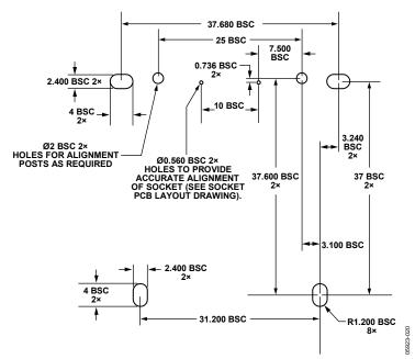
Figure 19. Printed Circuit Board Mounting Hole Pattern
