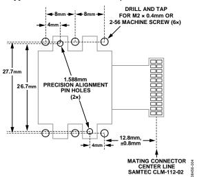
Figure 4. Example Hole Pattern for Machine Screw Placement
