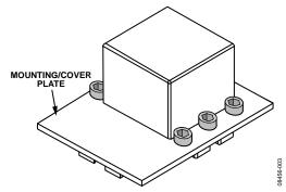
Figure 3. Cover Plate Mounting Example
