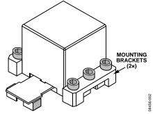
Figure 2. Bracket Mounting Example
