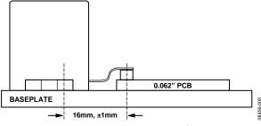
Figure 5. Dissimilar Mounting Surfaces
