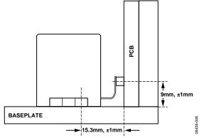
Figure 6. Orthogonal System Design Example
