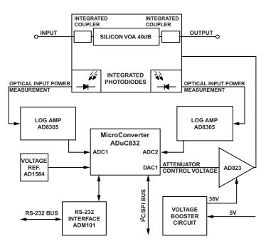
Figure 2. Overall DVOA Module Block Diagram
