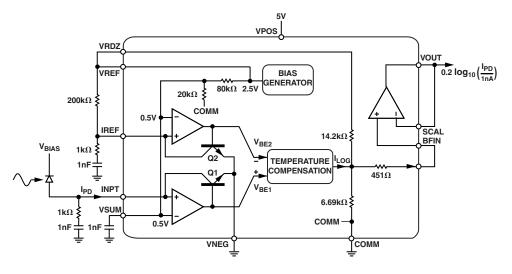
Figure 4. AD8305 Log Amp Block Diagram
