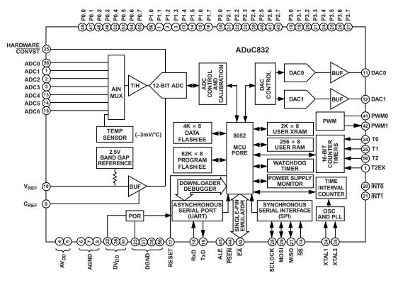
Figure 3. ADuC832 MicroConverter Block Diagram
