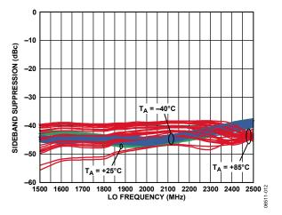
Figure 12. Sideband Suppression vs. f<sub>LO</sub> and Temperature Multiple Devices Shown
