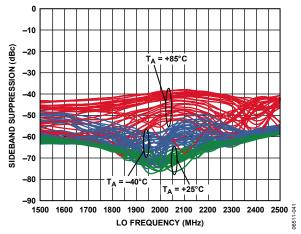
Figure 13. Sideband Suppression vs.  $f_{10}$  and Temperature after Nulling at 25  $^{\circ}$ C Multiple Devices Shown
