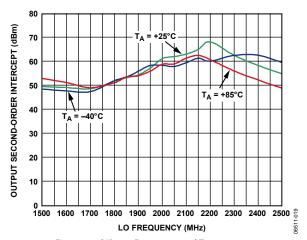
Figure 19. OIP2 vs. Frequency and Temperature
