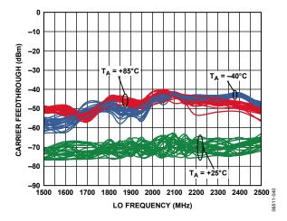
Figure 11. Carrier Feedthrough vs. f<sub>LO</sub> and Temperature after Nulling at 25°C Multiple Devices Shown
