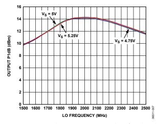
Figure 7. SSB Output P1dB Compression Point (OP1dB) vs.  $f_{L0}$  and Supply
