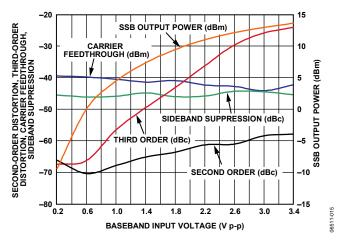
Figure 15. Second- and Third-Order Distortion, Carrier Feedthrough, Sideband Suppression, and SSB  $P_{\text{OUT}}$  vs. Baseband Differential Input Level ( $f_{\text{LO}} = 2150 \, \text{MHz}$ )
