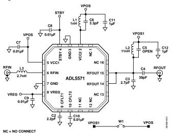
Figure 19. Basic Connections
