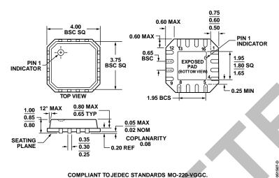
Figure 27. 16-Lead Lead Frame Chip Scale Package [LFCSP\_VQ] 4 mm × 4 mm Body, Very Thin Quad (CP-16-16)
