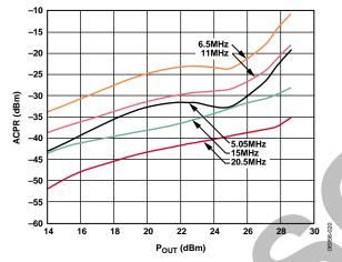
Figure 16. ACPR Measurement at 2.5 GHz
