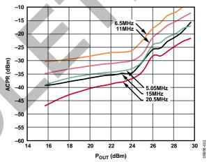
Figure 18. ACPR Measurement at 2.7 GHz
