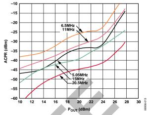
Figure 9. ACPR Measurement at 2.6 GHz
