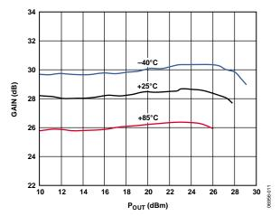
Figure 7. Gain vs.  $P_{OUT}$  at 2.6 GHz, Temperatures  $-40^{\circ}$ C,  $+25^{\circ}$ C, and  $+85^{\circ}$ C
