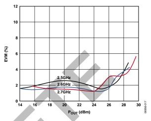
Figure 13. EVM vs. Pout at 2.5 GHz, 2.6 GHz, and 2.7 GHz
