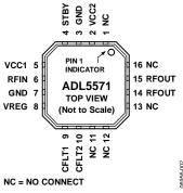
Figure 2. Pin Configuration
