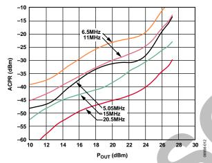
Figure 8. ACPR Measurement at 2.5 GHz
