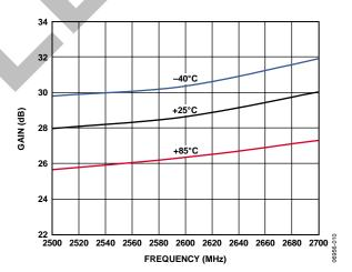
Figure 6. Gain vs. Frequency at  $P_{OUT} = 25$  dBm, Temperatures  $-40^{\circ}$ C,  $+25^{\circ}$ C, and  $+85^{\circ}$ C
