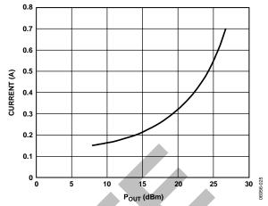
Figure 24. Burst Current vs.  $P_{OUT}$  at  $V_{CC}$  = 3.3 V, 64 QAM, 2350 MHz, 31% 802.16e OFDMA Signal
