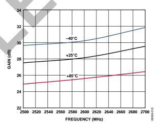
Figure 14. Gain vs. Frequency at  $P_{OUT} = 25$  dBm, Temperatures  $-40^{\circ}$ C,  $+25^{\circ}$ C, and  $+85^{\circ}$ C
