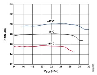
Figure 15. Gain vs.  $P_{OUT}$  at 2.6 GHz, Temperatures  $-40^{\circ}$ C,  $+25^{\circ}$ C, and  $+85^{\circ}$ C
