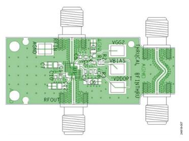
Figure 7. ADL9005-EVALZ Assembly Drawing (RFINTHRU and THRUCAL Not Installed)
