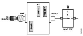
Figure 3. ADL9005-EVALZ Operation Using a Connectorized Bias Tee
