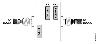
Figure 4. ADL9005-EVALZ Operation with  $V_{DD}$  Applied Through the VDDOPT SMT Test Point
