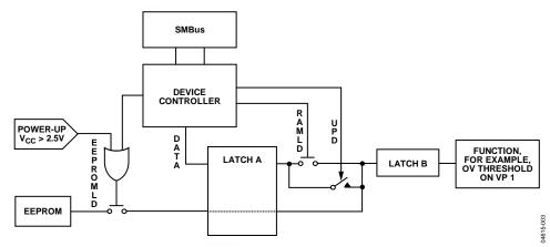
Figure 2. Configuration Update Flow Diagram
