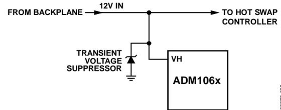
Figure 2. Implementing Transient Protection using a TVS
