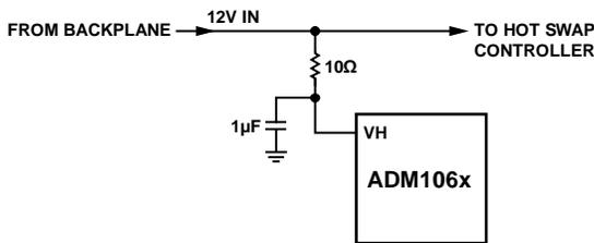
Figure 1. Using an RC Network to Provide Hot Swap Transient Protection
