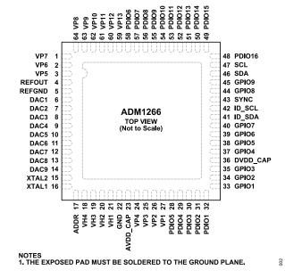
Figure 3. Pin Configuration
