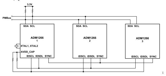
Figure 15. Setting Up Time Stamping in a Multidevice Setup
