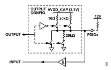
Figure 10. Programmable Driver Input/Output
