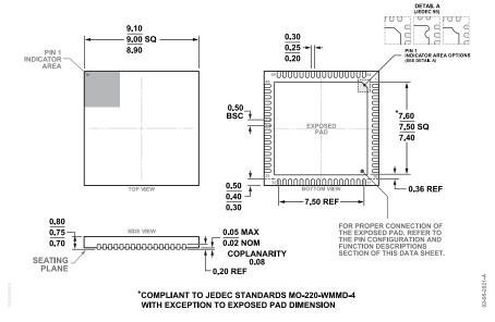
Figure 30. 64-Lead Lead Frame Chip Scale Package [LFCSP] 9 mm × 9 mm Body and 0.75 mm Package Height (CP-64-23) Dimensions shown in millimeters
