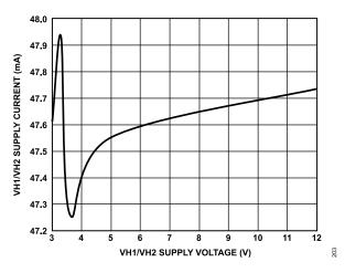
Figure 4. VH1/VH2 Current vs. VH1/VH2 Voltage with a 42 mA Load on AVDD CAP
