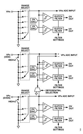
Figure 9. Supply Fault Detectors
