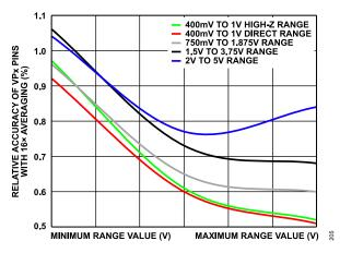
Figure 6. Relative Accuracy of VPx Pins with 16× Averaging (%) Across the Supply Fault Detector Range
