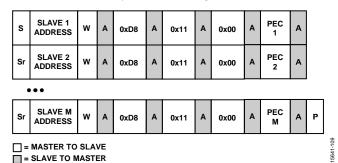
Figure 9. Group Command for Stopping a Sequence for Seamless Update
