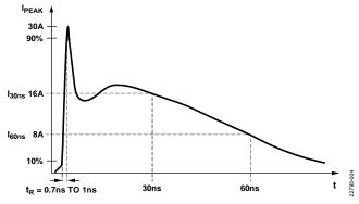
Figure 6. IEC 61000-4-2 ESD Waveform (8 kV)
