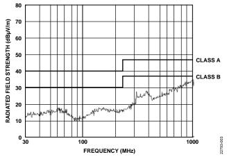
Figure 4. CISPR 32/EN 55032 Radiated Emissions Test Results
