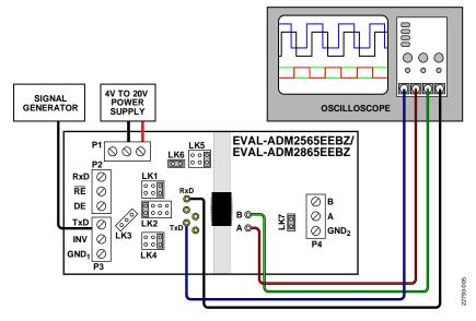
Figure 5. Half-Duplex RS-485 Loopback Test
