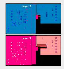
Figure 7. Embedded stitching capacitor.
