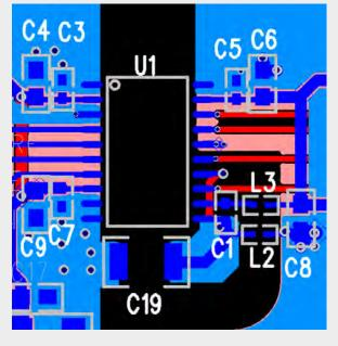
Figure 5. Placement of high voltage stitching capacitor.
