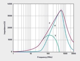
Figure 4. BLM15HD182SN1 impedance curve.
