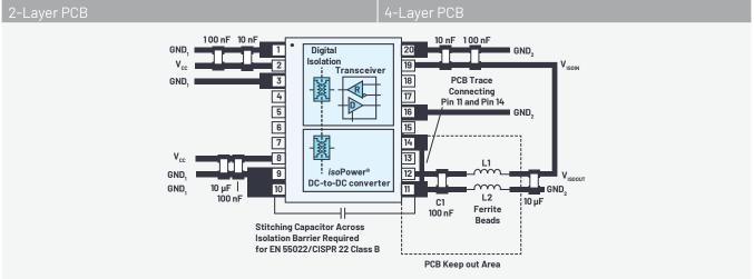
Figure 1. PCB decoupling for 2-layer and 4-layer PCB.
