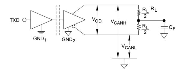
FIGURE 4. Driver voltage measurement.
