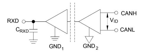
FIGURE 5. Receiver voltage measurement.
