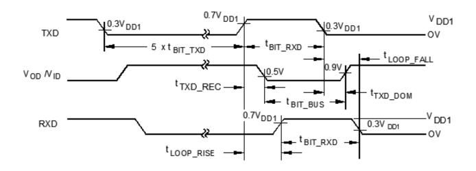
FIGURE 6. <u>Transceiver timing diagram</u>.
