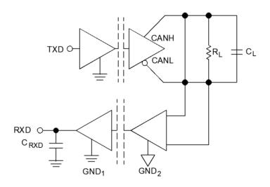
FIGURE 8. Switching characteristics measurements.
