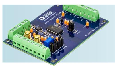
The ADM3055E family of CAN FD transceivers meets EN 55032 Class B without stitching capacitance on elegant 2-layer evaluation boards.
