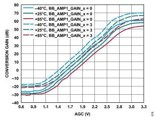
Figure 77. Conversion Gain vs. AGC, LO = 17 GHz, Maximum Gain (Minimum Input Power) at Various Temperatures and Various BB\_AMP1\_GAIN\_x
