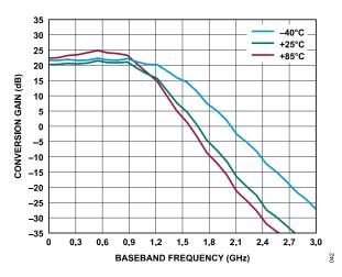
Figure 42. Bypass, SPI-Selectable LPFs, Conversion Gain vs. Baseband Frequency at Various Temperatures
