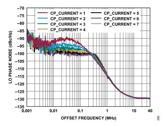
Figure 59. LO Phase Noise vs. Offset Frequency, CP\_CURRENT = 1 to 7, LO = 17 GHz, and SI\_VCO\_CORE = 1
