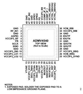
Figure 2. Pin Configuration
