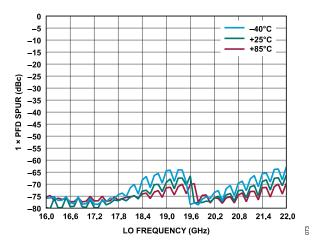
Figure 72. 1 × PFD Spur vs. LO Frequency at Various Temperatures, Spur Referred to the Main I Channel and Q Channel Output Frequency
