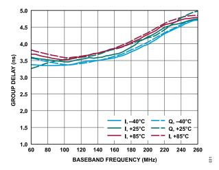
Figure 31. 250 MHz, SPI-Selectable Baseband LPF, Group Delay vs. Baseband Frequency at Various Temperatures and the I and Q Channels
