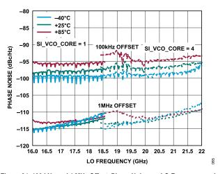
Figure 64. 100 kHz and 1 MHz Offset, Phase Noise vs. LO Frequency and at Various Temperatures, CP\_CURRENT = 4
