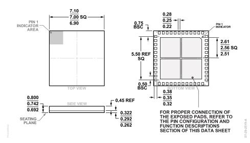
Figure 89. 48-Terminal Land Grid Array [LGA] (CC-48-5) Dimensions Shown in Millimeters
