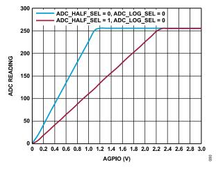
Figure 50. ADC Reading vs. AGPIO for ADC\_LOG\_SEL = 0
