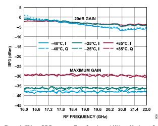
Figure 9. IIP3 vs. RF Frequency, Tone Spacing = 1 MHz, at Maximum Gain (Minimum Input Power) and 20 dB Gain (Maximum Input Power) at Various Temperatures and I and Q Channels
