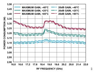
Figure 21. Power Consumption vs. RF Frequency for Maximum Gain (Minimum Input Power) and 20 dB Gain (Maximum Input Power) at Various Temperatures
