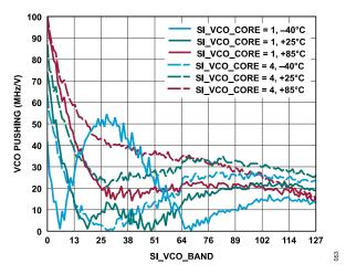
Figure 53. VCO Pushing vs. SI\_VCO\_BAND, Open Loop, VTUNE = 1.5 V, at Various Temperatures, SI\_VCO\_CORE = 1 and = 4
