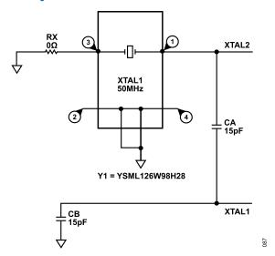
Figure 86. External Circuitry for Crystal Oscillator
