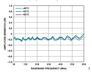
Figure 39. 500 MHz, SPI-Selectable LPF, Amplitude Mismatch vs. Baseband Frequency at Various Temperatures
