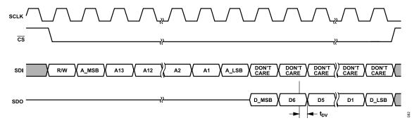
Figure 81. Timing Diagram for Analog Devices Standard SPI Register Read, 4-Wire Mode
