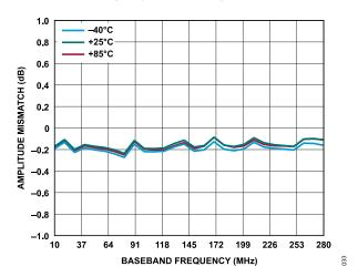
Figure 33. 250 MHz, SPI-Selectable Baseband LPF, Amplitude Mismatch vs. Baseband Frequency at Various Temperatures
