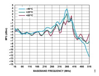
Figure 36. 500 MHz, SPI-Selectable LPF, IIP3 vs. Baseband Frequency at Various Temperatures at 20 dB Gain (Maximum Input Power)
