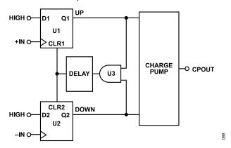
Figure 87. PFD and Charge Pump Simplified Schematic
