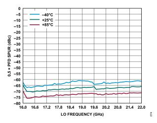
Figure 73. 0.5 × PFD Spur vs. LO Frequency at Various Temperatures, Spur Referred to the Main I Channel and Q Channel Output Frequency
