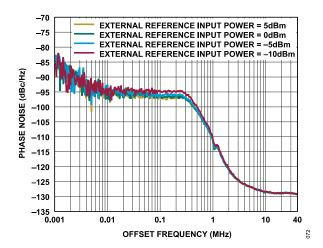
Figure 71. Phase Noise vs. Offset Frequency over the External Reference Input Power, LO = 21 GHz
