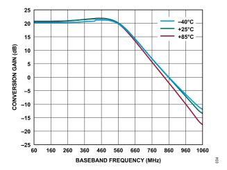
Figure 34. 500 MHz, SPI-Selectable LPF Frequency Response, Conversion Gain vs. Baseband Frequency at Various Temperatures
