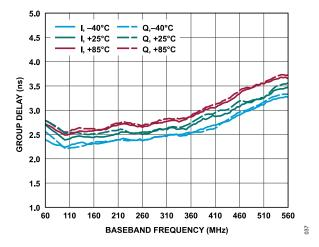
Figure 37. 500 MHz, SPI-Selectable LPF, Group Delay vs. Baseband Frequency at Various Temperatures and the I and Q Channels
