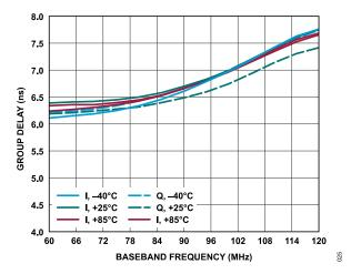
Figure 25. 125 MHz, SPI-Selectable Baseband LPF, Group Delay vs. Baseband Frequency at Various Temperatures and the I and Q Channels
