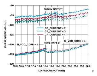
Figure 67. 100 kHz and 1 MHz Offset, Phase Noise vs. LO Frequency at Various Temperatures, CP \_CURRENT = 2, 3, and 4
