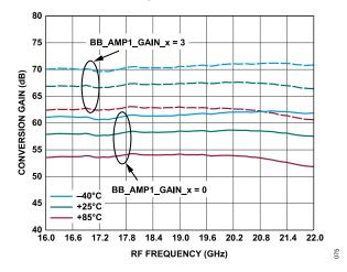
Figure 74. Conversion Gain vs. RF Frequency at Maximum Gain (Minimum Input Power) at Various Temperatures and Various BB\_AMP1\_GAIN\_x
