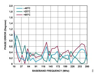
Figure 32. 250 MHz, SPI-Selectable Baseband LPF, Phase Error vs. Baseband Frequency at Various Temperatures
