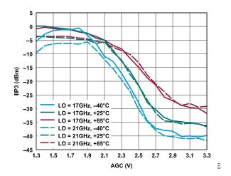
Figure 11. IIP3 vs. AGC, LO = 17 GHz and 21 GHz at Various Temperatures
