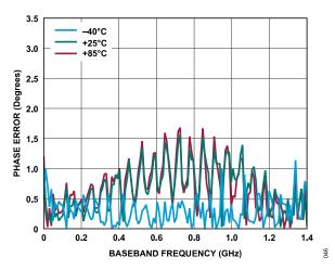
Figure 46. Bypass, SPI-Selectable LPFs, Phase Error vs. Baseband Frequency at Various Temperatures
