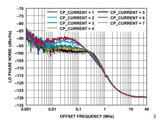
Figure 61. LO Phase Noise vs. Offset Frequency, CP\_CURRENT = 1 to 7, LO = 19 GHz, and SI\_VCO\_CORE = 4
