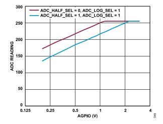
Figure 49. ADC Reading vs. AGPIO for ADC\_LOG\_SEL = 1
