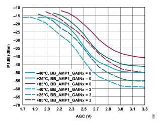
Figure 79. IP1dB vs. AGC, LO = 21 GHz Various Temperatures
