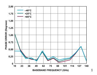
Figure 26. 125 MHz, SPI-Selectable Baseband LPF, Phase Error vs. Baseband Frequency at Various Temperatures
