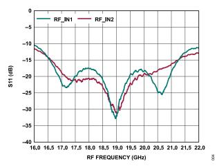
Figure 4. Input Return Loss (S11) vs. RF Frequency for RF\_IN1 and RF\_IN2
