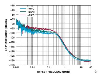
Figure 56. LO Phase Noise vs. Offset Frequency at 17.1 GHz and at Various Temperatures, CP\_CURRENT = 4 and SI\_VCO\_CORE = 1
