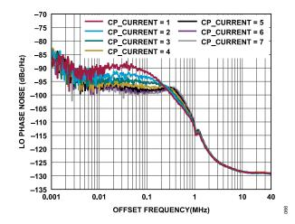
Figure 65. LO Phase Noise vs. Offset Frequency, CP\_CURRENT = 1 to 7, LO = 21 GHz, and SI\_VCO\_CORE = 1
