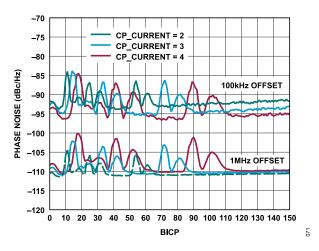
Figure 70. 100 kHz and 1 MHz Offset, Phase Noise vs. BICP, CP\_CURRENT = 2, 3, and 4 and LO = 21 GHz
