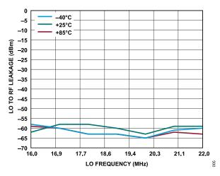
Figure 5. LO to RF Leakage vs. LO Frequency at Various Temperatures
