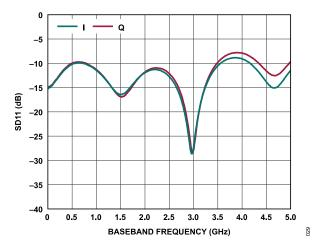
Figure 29. 250 MHz, SPI-Selectable Baseband LPF, I and Q SD11 vs. Baseband Frequency
