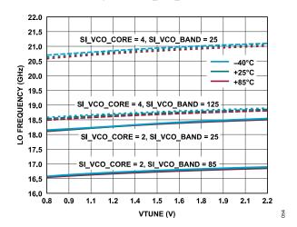
Figure 54. LO Frequency vs. VTUNE over Temperature, Four Bands (Two Bands for VCO Core 1 and Two Bands for VCO Core 2)
