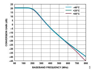
Figure 28. 250 MHz, SPI-Selectable Baseband LPF Frequency Response, Conversion Gain vs. Baseband Frequency at Various Temperatures
