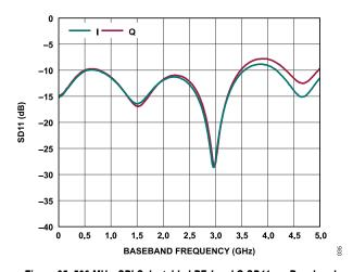
Figure 35. 500 MHz, SPI-Selectable LPF, I and Q SD11 vs. Baseband Frequency
