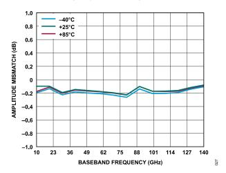
Figure 27. 125 MHz, SPI-Selectable Baseband LPF, Amplitude Mismatch vs. Baseband Frequency at Various Temperatures
