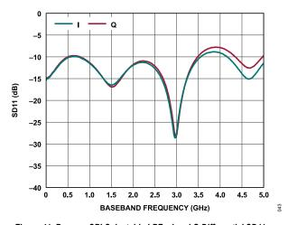
Figure 41. Bypass, SPI-Selectable LPFs, I and Q Differential SD11 vs.
