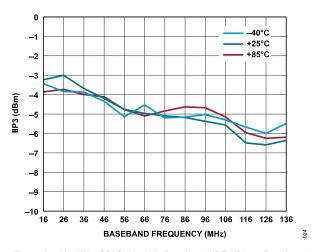
Figure 24. 125 MHz, SPI-Selectable Baseband LPF, IIP3 vs. Baseband Frequency at Various Temperatures at 20 dB Gain (Maximum Input Power)
