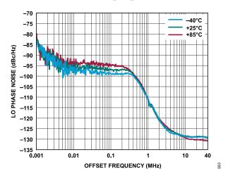
Figure 62. LO Phase Noise vs. Offset Frequency at 21 GHz and at Various Temperatures, CP\_CURRENT = 4 and SI\_VCO\_CORE = 4
