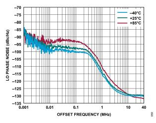
Figure 58. LO Phase Noise vs. Offset Frequency at 18.6 GHz and at Various Temperatures, CP\_CURRENT = 4 and SI\_VCO\_CORE = 4
