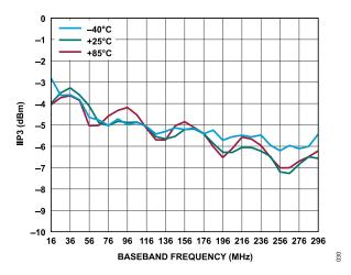
Figure 30. 250 MHz, SPI-Selectable Baseband LPF, IIP3 vs. Baseband Frequency at Various Temperatures at 20 dB Gain (Maximum Input Power)
