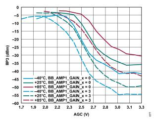
Figure 76. IIP3 vs. AGC, LO = 21 GHz at Maximum Gain (Minimum Input Power) at Various Temperatures and Various BB\_AMP1\_GAIN\_x Settings
