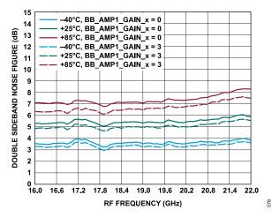
Figure 75. Double Sideband Noise Figure vs. RF Frequency at Maximum Gain (Minimum Input Power) at Various Temperatures and Various BB\_AMP1\_GAIN\_x Settings
