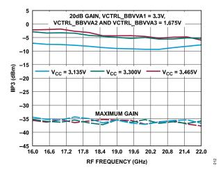
Figure 12. IIP3 vs. RF Frequency at Maximum Gain (Minimum Input Power) and 20 dB Gain (Maximum Input Power) at Various Supply Voltages (±5)
