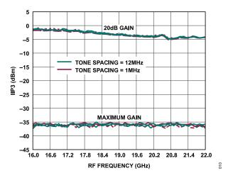
Figure 10. IIP3 vs. RF Frequency, Tone Spacing = 12 MHz and 1 MHz at Maximum Gain (Minimum Input Power) and 20 dB Gain (Maximum Input Power)
