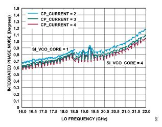
Figure 66. Integrated Phase Noise, 1 kHz to 10 MHz vs. LO Frequency, CP CURRENT = 2, 3, and 4
