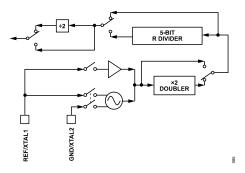
Figure 84. Reference Input Stage
