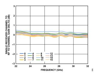
Figure 56. Single Receiver Channel to RF to Channel Gain Delta vs.
