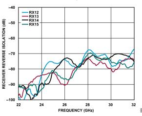
Figure 75. Receiver Reverse Isolation vs. Frequency for RX12 to RX15
