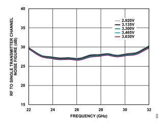
Figure 27. RF to Single Transmitter Channel Noise Figure vs. Frequency at Various Supply Voltages at Maximum Gain
