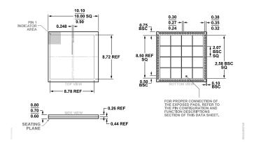
Figure 96. 72-Terminal Land Grid Array [LGA] (CC-72-3) Dimensions shown in millimeters
