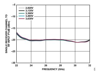
Figure 64. Single Receiver Channel to RF Input P1dB vs. Frequency at Various Supply Voltages at Maximum Gain
