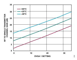
Figure 8. RF to Single Transmitter Channel Gain vs. DVGA 1 Setting from 0 to 35 over Various Temperatures at 27 GHz
