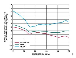
Figure 54. Single Receiver Channel to RF Phase Error vs. Frequency for Peak, Average, and RMS Error
