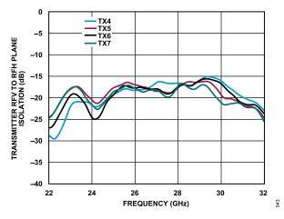
Figure 37. Transmitter RFV to RFH Plane Isolation vs. Frequency for Transmitter 2 (TX4), Transmitter 5 (TX5), Transmitter 6 (TX6), and Transmitter 7 (TX7)
