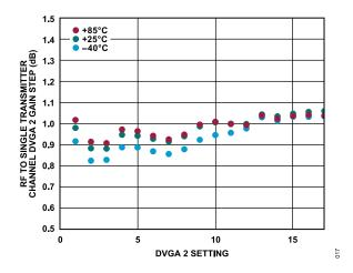
Figure 11. RF to Single Transmitter Channel DVGA 2 Gain Step vs. DVGA 2 Setting from 0 to 17 over Various Temperatures at 27 GHz
