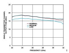
Figure 87. Single Transmitter Channel Output P1dB vs. Frequency at Various Power Modes, Maximum Gain
