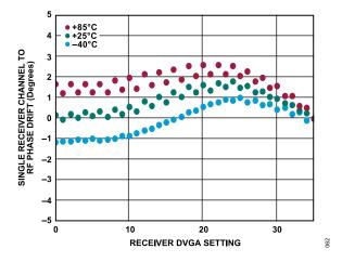
Figure 52. Single Receiver Channel to RF Phase Drift Setting from 0 to 35 over Various Temperatures at 27 GHz
