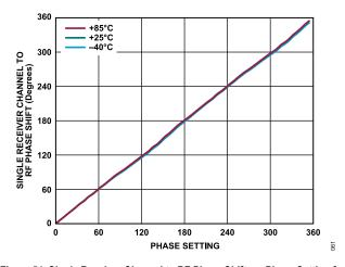
Figure 51. Single Receiver Channel to RF Phase Shift vs. Phase Setting from 0° to 360° over Various Temperatures at 27 GHz, Set to Maximum Gain
