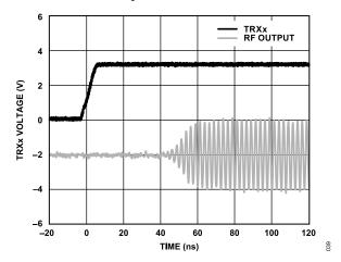
Figure 33. Receiver to Transmitter Mode Switching Time
