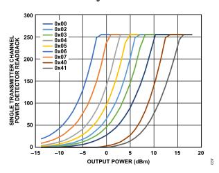
Figure 31. Single Transmitter Channel Power Detector Readback vs. Output Power at Various Detector Range Settings at 27 GHz, Set to Maximum Gain
