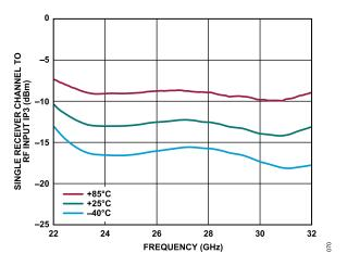
Figure 60. Single Receiver Channel to RF Input IP3 vs. Frequency at Various
