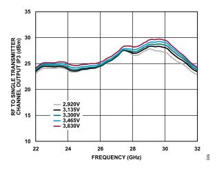
Figure 23. RF to Single Transmitter Channel Output IP3 vs. Frequency at Various Supply Voltages at Maximum Gain
