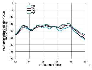
Figure 36. Transmitter RFV to RFH Plane Isolation vs. Frequency for Transmitter 0 (TX0), Transmitter 1 (TX1), Transmitter 2 (TX2), and Transmitter 3 (TX3)
