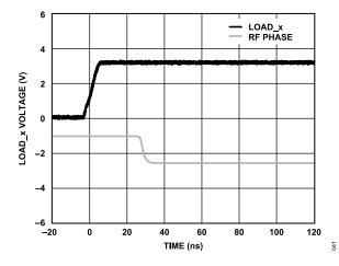
Figure 35. RF Phase Settling Time
