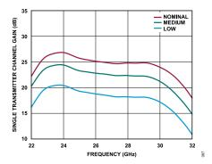
Figure 86. Single Transmitter Channel Gain vs. Frequency at Various Power Modes, Maximum Gain
