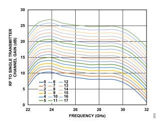
Figure 7. RF to Single Transmitter Channel Gain vs. Frequency at Various DVGA 2 Settings from 0 to 17
