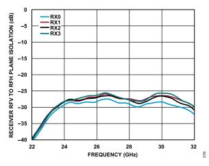
Figure 68. Receiver RFV to RFH Plane Isolation vs. Frequency for Receiver 0 (RX0), Receiver 1 (RX1), Receiver 2 (RX2), and Receiver 3 (RX3)
