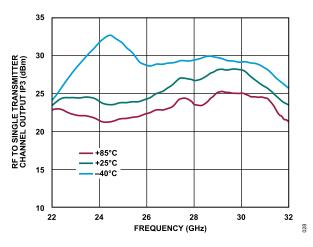
Figure 22. RF to Single Transmitter Channel Output IP3 vs. Frequency at Various Temperatures at Maximum Gain
