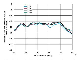
Figure 38. Transmitter RFV to RFH Plane Isolation vs. Frequency for Transmitter 8 (TX8), Transmitter 9 (TX9), Transmitter 10 (TX10), and Transmitter 11 (TX11)
