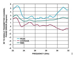
Figure 16. RF to Single Transmitter Channel Phase Error vs. Frequency for Peak, Average, and RMS Error
