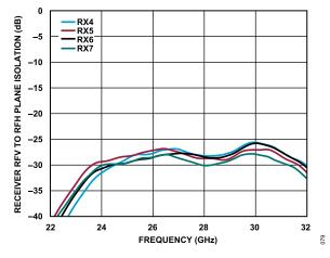
Figure 69. Receiver RFV to RFH Plane Isolation vs. Frequency for Receiver 4 (RX4), Receiver 5 (RX5), Receiver 6 (RX6), and Receiver 7 (RX7)
