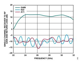
Figure 45. Single Channel Receiver to RF Gain and Return Loss vs.
