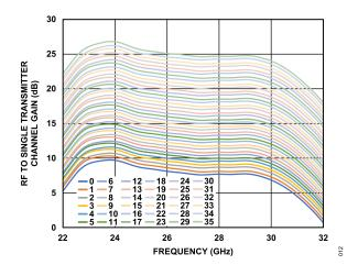
Figure 6. RF to Single Transmitter Channel Gain vs. Frequency at Various DVGA 1 Settings from 0 to 35
