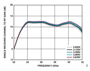
Figure 46. Single Receiver Channel to RF Gain vs. Frequency at Various Supply Voltages at Maximum Gain
