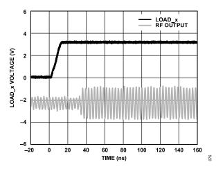
Figure 66. Gain Settling Time
