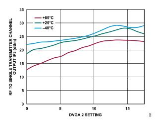
Figure 25. RF to Single Transmitter Channel Output IP3 vs. DVGA 2 Setting from 0 to 17 over Various Temperatures at 27 GHz
