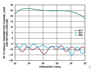
Figure 5. RF to Single Transmitter Channel Gain and Return Loss vs. Frequency at Maximum Gain
