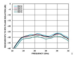
Figure 71. Receiver RFV to RFH Plane Isolation vs. Frequency for Receiver 12 (RX12), Receiver 13 (RX13), Receiver (RX14), and Receiver 15 (RX15)
