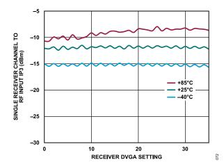
Figure 62. Single Receiver Channel to RF Input IP3 vs. Receiver DVGA Setting from 0 to 35 over Various Temperatures at 27 GHz
