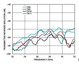
Figure 42. Transmitter Reverse Isolation vs. Frequency for TX8 to TX11
