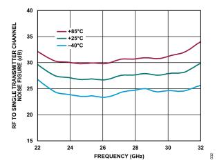
Figure 26. RF to Single Transmitter Channel Noise Figure vs. Frequency at Various Temperatures at Maximum Gain
