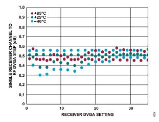
Figure 49. Single Receiver Channel to RF DVGA Step vs. Receiver DVGA Setting from 0 to 35 over Various Temperatures at 27 GHz
