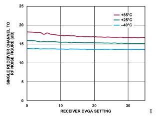
Figure 59. Single Receiver Channel to RF Noise Figure vs. Receiver DVGA Setting from 0 to 35 over Various Temperatures at 27 GHz
