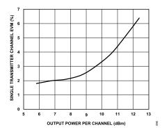
Figure 95. Single Transmitter Channel EVM vs. Output Power Per Channel at Maximum Gain
