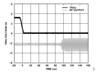
Figure 65. Transmitter to Receiver Mode Switching Time
