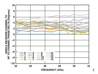
Figure 55. Single Receiver Channel to RF to Channel Phase Delta vs. Frequency at Maximum Gain, Where Numbers in Legend Are Channel Numbers
