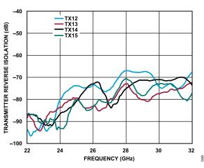
Figure 43. Transmitter Reverse Isolation vs. Frequency for TX12 to TX15
