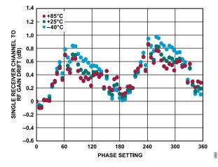
Figure 50. Single Receiver Channel to RF Gain Drift vs. Phase Setting from 0° to 360° over Temperature at 27 GHz, Set to Maximum Gain
