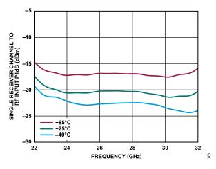
Figure 63. Single Receiver Channel to RF Input P1dB vs. Frequency at Various Temperatures at Maximum Gain
