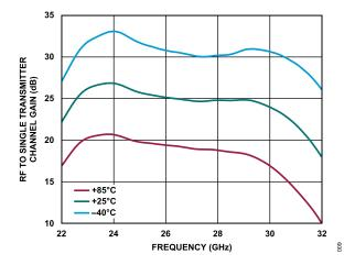
Figure 3. RF to Single Transmitter Channel Gain vs. Frequency at Various Temperatures at Maximum Gain
