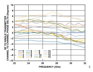
Figure 17. RF to Single Transmitter Channel to Channel Phase Delta vs. Frequency at Maximum Gain, Where Numbers in Legend Are Channel Numbers
