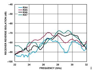
Figure 73. Receiver Reverse Isolation vs. Frequency for RX4 to RX7
