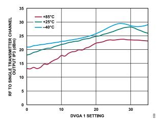
Figure 24. RF to Single Transmitter Channel Output IP3 vs. DVGA 1 Setting from 0 to 35 over Various Temperatures at 27 GHz
