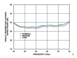
Figure 89. Single Transmitter Channel Noise Figure vs. Frequency at Various Power Modes, Maximum Gain
