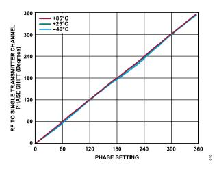
Figure 13. RF to Single Transmitter Channel Phase Shift vs. Phase Setting from 0° to 360° over Various Temperatures at 27 GHz, Set to Maximum Gain
