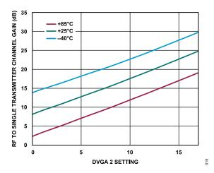
Figure 9. RF to Single Transmitter Channel Gain vs. DVGA 2 Setting from 0 to 17 over Various Temperatures at 27 GHz
