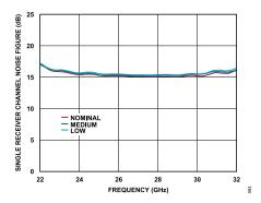
Figure 92. Single Receiver Channel Noise Figure vs. Frequency at Various Temperatures, Maximum Gain
