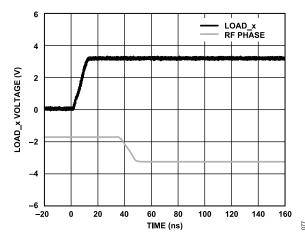
Figure 67. RF Phase Settling Time
