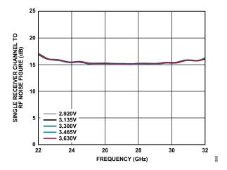
Figure 58. Single Receiver Channel to RF Noise Figure vs. Frequency at Various Supply Voltages at Maximum Gain
