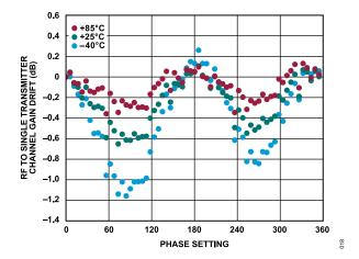
Figure 12. RF to Single Transmitter Channel Gain Drift vs. Phase Setting from 0° to 360° over Temperature at 27 GHz, Set to Maximum Gain
