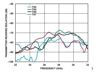
Figure 41. Transmitter Reverse Isolation vs. Frequency for TX4 to TX7
