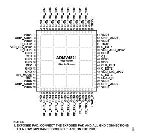
Figure 2. Pin Configuration
