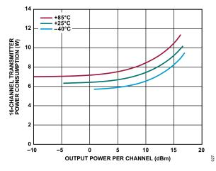
Figure 21. 16-Channel Transmitter Power Consumption vs. Output Power per Channel at Various Temperatures at Maximum Gain
