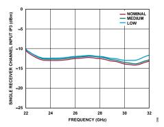
Figure 94. Single Receiver Channel Input IP3 vs. Frequency at Various Temperatures, Maximum Gain
