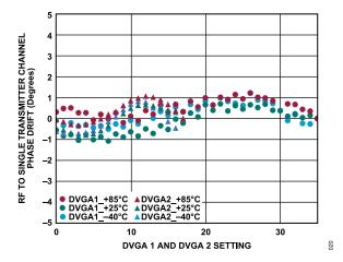
Figure 14. RF to Single Transmitter Channel Phase Drift vs. DVGA 1 Setting from 0 to 35 and DVGA 2 Setting from 0 to 17, over Various Temperatures at 27 GHz
