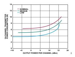
Figure 90. 16-Channel Transmitter Power Consumption vs. Output Power per Channel, Maximum Gain
