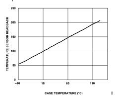
Figure 79. Temperature Sensor Readback vs. Case Temperature
