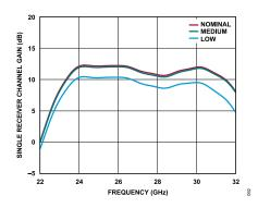
Figure 91. Single Receiver Channel Gain vs. Frequency at Various Temperatures, Maximum Gain
