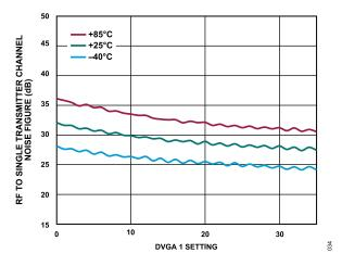
Figure 28. RF to Single Transmitter Channel Noise Figure vs. DVGA 1 Setting from 0 to 35 over Various Temperatures at 27 GHz
