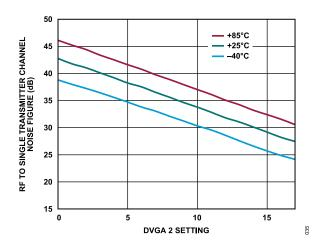
Figure 29. RF to Single Transmitter Channel Noise Figure vs. DVGA 2 Setting from 0 to 17 over Various Temperatures at 27 GHz
