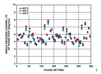
Figure 53. Single Receiver Channel to RF Phase Step vs. Phase Setting from 0° to 360° over Various Temperatures at 27 GHz, Set to Maximum Gain, Nominal Step = 5.625°
