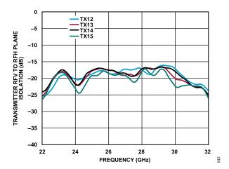
Figure 39. Transmitter RFV to RFH Plane Isolation vs. Frequency for Transmitter 12 (TX12), Transmitter 13 (TX13), Transmitter 14 (TX14), and Transmitter 15 (TX15)
