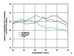
Figure 88. Single Transmitter Channel Output IP3 vs. Frequency at Various Power Modes, Maximum Gain
