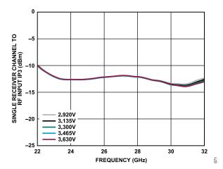
Figure 61. Single Receiver Channel to RF Input IP3 vs. Frequency at Various Supply Voltages at Maximum Gain
