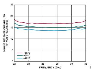
Figure 57. Single Receiver Channel to RF Noise Figure vs. Frequency at Various Temperatures at Maximum Gain
