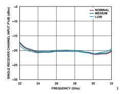
Figure 93. Single Receiver Channel Input P1dB vs. Frequency at Various Temperatures, Maximum Gain
