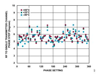
Figure 15. RF to Single Transmitter Channel Phase Step vs. Phase Setting from 0° to 360° over Various Temperatures at 27 GHz, Set to Maximum Gain, Nominal Step 5.625°
