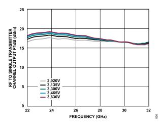
Figure 20. RF to Single Transmitter Channel Output P1dB vs. Frequency at Various Supply Voltages at Maximum Gain
