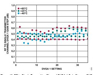
Figure 10. RF to Single Transmitter Channel DVGA 1 Gain Step vs. DVGA 1 Setting from 0 to 35 over Various Temperatures at 27 GHz
