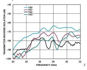
Figure 40. Transmitter Reverse Isolation vs. Frequency for TX0 to TX3
