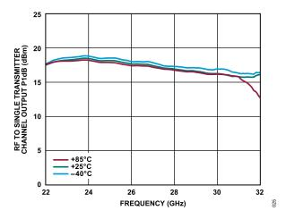
Figure 19. RF to Single Transmitter Channel Output P1dB vs. Frequency at Various Temperatures at Maximum Gain
