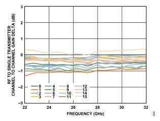
Figure 18. RF to Single Transmitter Channel to Channel Gain Delta vs.
