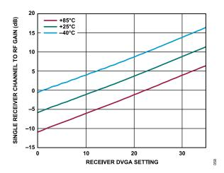
Figure 48. Single Receiver Channel to RF Gain vs. Receiver DVGA Setting from 0 to 35 over Various Temperatures at 27 GHz
