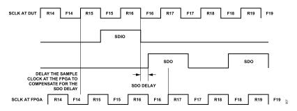
Figure 85. Using a Delayed SCLK
