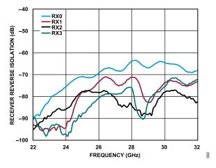
Figure 72. Receiver Reverse Isolation vs. Frequency for RX0 to RX3
