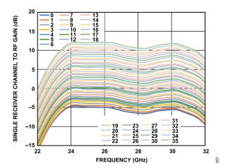
Figure 47. Single Receiver Channel to RF Gain vs. Frequency at Various Receiver DVGA Settings from 0 to 35
