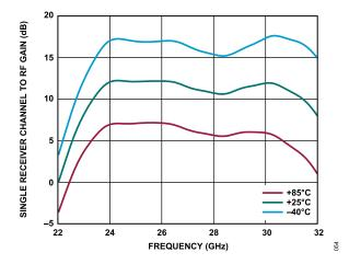
Figure 44. Single Receiver Channel to RF Gain vs. Frequency at Various Temperatures at Maximum Gain
