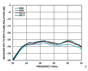
Figure 70. Receiver RFV to RFH Plane Isolation vs. Frequency for Receiver 8 (RX8), Receiver 9 (RX9), Receiver 10 (RX10), and Receiver 11 (RX11)
