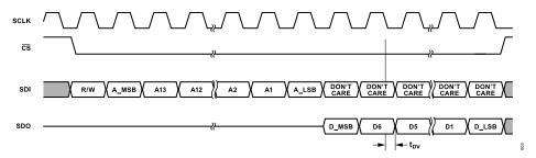
Figure 81. Timing Diagram for Standard SPI Register Read, 4-Wire Mode,
