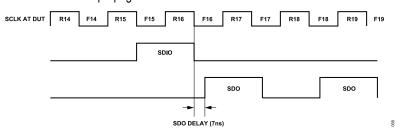
Figure 83. SDO Delay Timing Diagram
