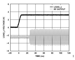
Figure 34. Gain Settling Time
