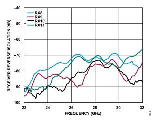
Figure 74. Receiver Reverse Isolation vs. Frequency for RX8 to RX11
