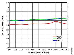
Figure 22. Output P1dB vs. RF Frequency over Temperature, Gain = 23.5 dB
