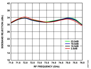
Figure 54. Sideband Rejection vs. RF Frequency at Various Gains
