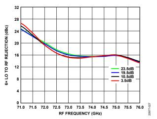
Figure 27. 6× LO to RF Rejection vs. RF Frequency at Various Gains
