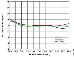
Figure 61.  $6 \times$  LO Rejection vs. RF Frequency over Temperature, Gain = 23.5 dB
