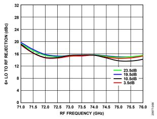
Figure 66. 6× LO to RF Rejection vs. RF Frequency at Various Gains
