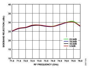
Figure 43. Sideband Rejection vs. RF Frequency at Various Gains
