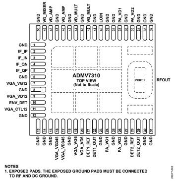
Figure 2. Pin Configuration
