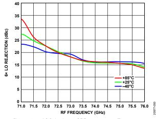
Figure 50.  $6 \times$  LO Rejection vs. RF Frequency over Temperature, Gain = 23.5 dB
