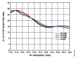
Figure 44. 6× LO to RF Rejection vs. RF Frequency at Various Gains
