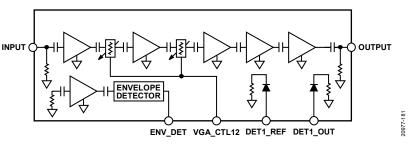
Figure 81. Variable Gain Amplifier Circuit Architecture
