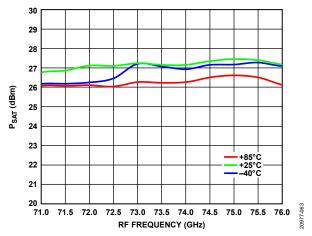
Figure 63. P<sub>SAT</sub> vs. RF Frequency over Temperature, Gain = 23.5 dB
