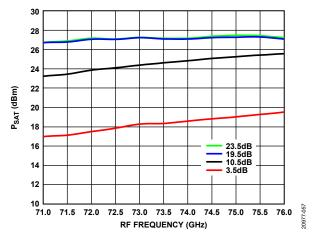
Figure 57. P<sub>SAT</sub> vs. RF Frequency at Various Gains
