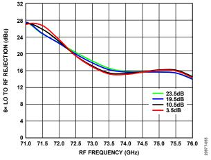
Figure 55. 6× LO to RF Rejection vs. RF Frequency at Various Gains
