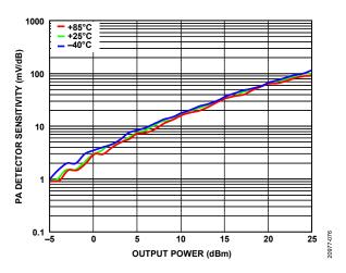
Figure 75. PA Detector Sensitivity vs. Output Power over Temperature,  $RF = 71~\mathrm{GHz}$
