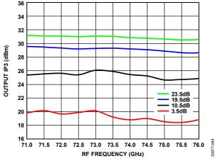
Figure 64. Output IP3 vs. RF Frequency at Various Gains
