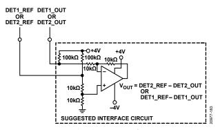
Figure 83. Typical Application Circuit for Power Detector
