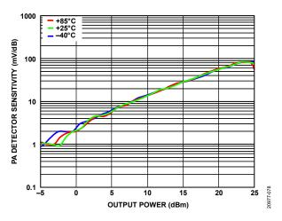
Figure 77. PA Detector Sensitivity vs. Output Power over Temperature,  $RF = 76\,\mathrm{GHz}$
