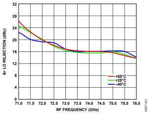
Figure 21.  $6 \times$  LO Rejection vs. RF Frequency over Temperature, Gain = 23.5 dB
