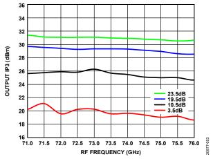
Figure 53. Output IP3 vs. RF Frequency at Various Gains
