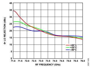
Figure 39.  $6 \times$  LO Rejection vs. RF Frequency over Temperature, Gain = 23.5 dB
