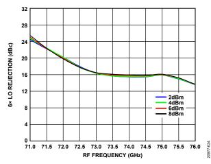
Figure 24.  $6 \times$  LO Rejection vs. RF Frequency over LO Power, Gain = 23.5 dB
