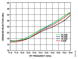
Figure 65. Sideband Rejection vs. RF Frequency at Various Gains
