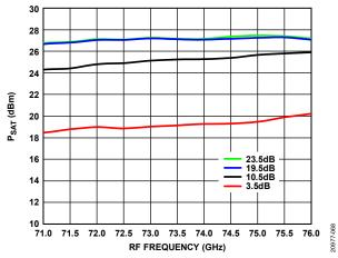
Figure 68. P<sub>SAT</sub> vs. RF Frequency at Various Gains
