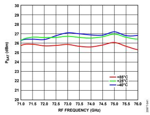
Figure 41. P<sub>SAT</sub> vs. RF Frequency over Temperature, Gain = 23.5 dB
