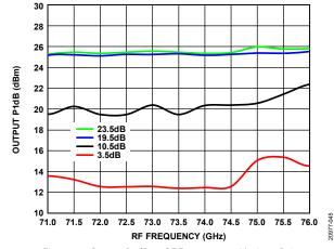
Figure 45. Output P1dB vs. RF Frequency at Various Gains
