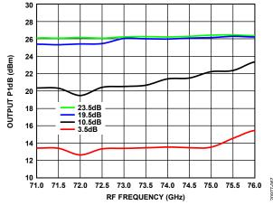
Figure 67. Output P1dB vs. RF Frequency at Various Gains
