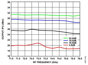
Figure 42. Output IP3 vs. RF Frequency at Various Gains
