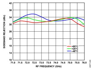
Figure 49. Sideband Rejection vs. RF Frequency over Temperature, Gain = 23.5 dB
