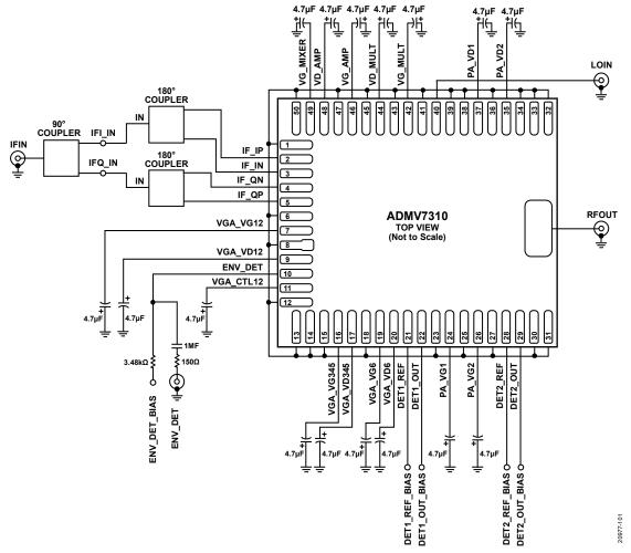
Figure 86. Typical Application Circuit
