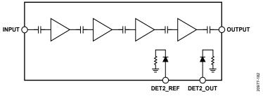
Figure 82. Power Amplifier Circuit Architecture
