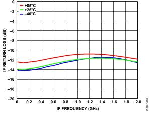
Figure 80. IF Return Loss vs. IF Frequency over Temperature
