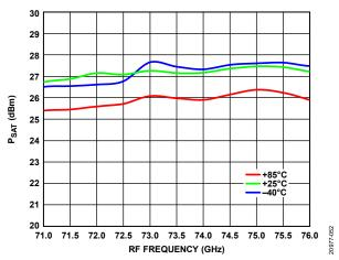
Figure 52. P<sub>SAT</sub> vs. RF Frequency over Temperature, Gain = 23.5 dB
