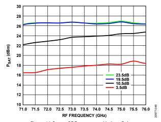
Figure 46.  $P_{SAT}$  vs. RF Frequency at Various Gains
