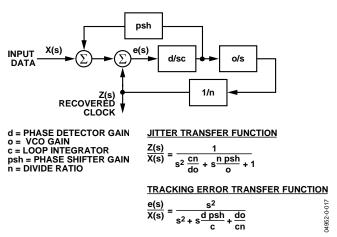
Figure 13. ADN2815 PLL/DLL Architecture
