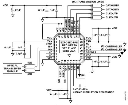
Figure 19. Typical ADN2815 Applications Circuit
