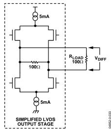
Figure 4. Differential Output Stage
