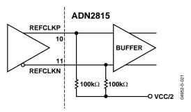
Figure 16. Differential REFCLK Configuration
