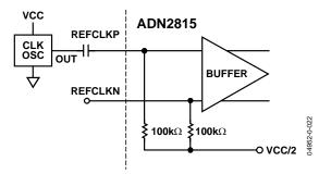
Figure 17. Single-Ended REFCLK Configuration
