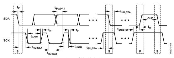
Figure 10.  $I^2C$  Port Timing Diagram
