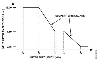
Figure 12. SONET Jitter Tolerance Mask
