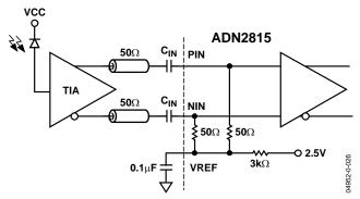
Figure 20. ADN2815 AC-Coupled Input Configuration
