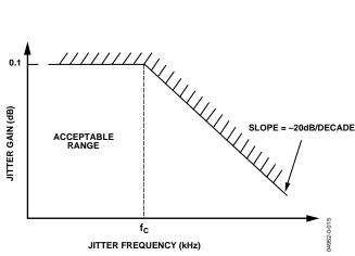
Figure 11. Jitter Transfer Curve
