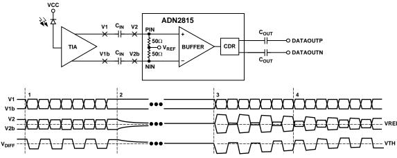
V<sub>DIFF</sub> = V2–V2b VTH = ADN2815 QUANTIZER THRESHOLD
