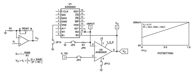
Figure 6. Noninverting Linear Gain
