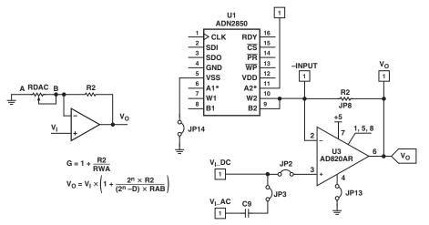
Figure 7. Noninverting Exponential Gain
