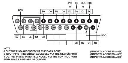
Figure 11. Parallel Port Connector Configuration (For VB Program Developers Only)
