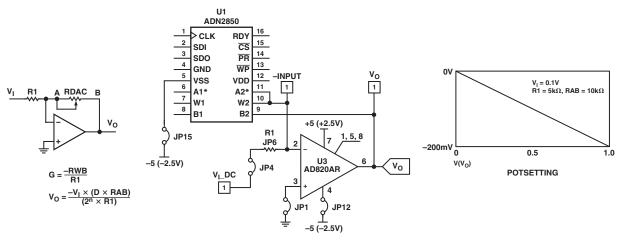
Figure 4. Inverting Linear Gain and Attenuator
