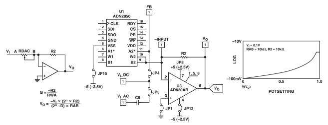
Figure 5. Inverting Exponential Gain and Attenuator
