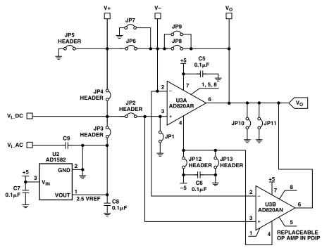
Figure 3. Evaluation Board Schematic
