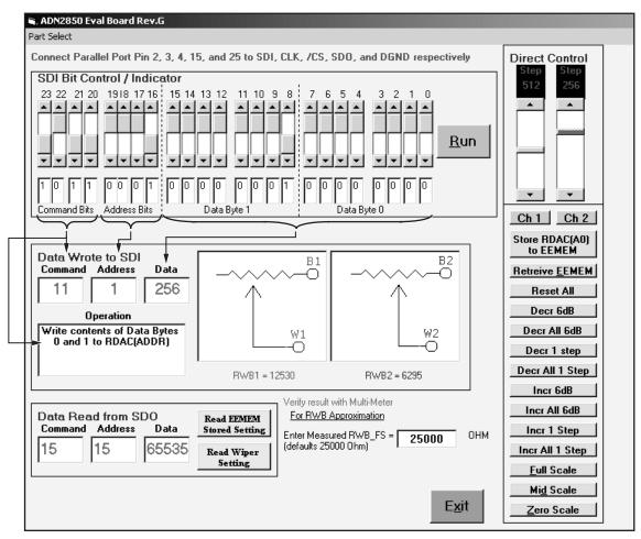
Figure 2. ADN2850 Software Graphical Interface
