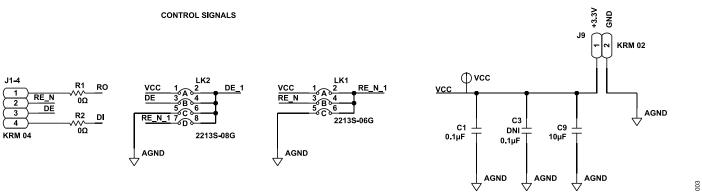
Figure 3. EVAL-ADN4693E-1EBZ Schematic
