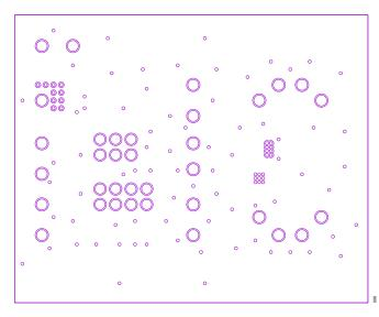
Figure 6. EVAL-ADN4693E-1EBZ Internal Layer 2 (GND)
