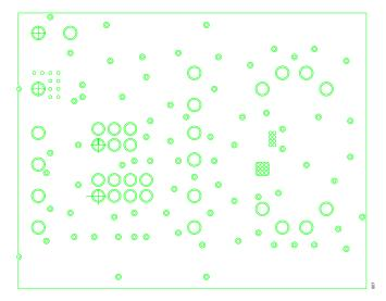
Figure 7. EVAL-ADN4693E-1EBZ Internal Layer 3 (VCC)
