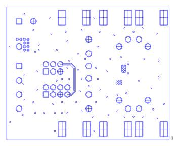
Figure 8. EVAL-ADN4693E-1EBZ Solder Side
