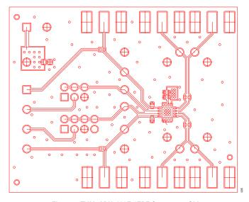
Figure 5. EVAL-ADN4693E-1EBZ Component Side
