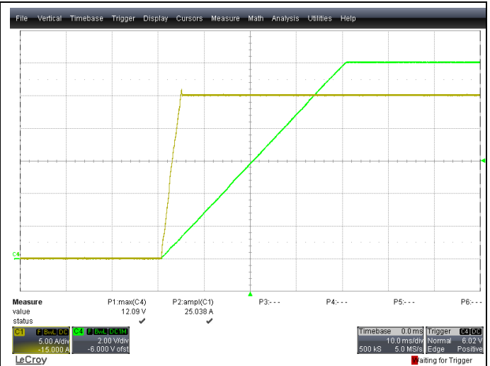
Figure 12 - Startup at 60VDC, 25A load (2A/us slew rate) Green trace: Output voltage, 2V/div, 10ms/div Yellow trace: Load current, 5A/div, 10ms/div
