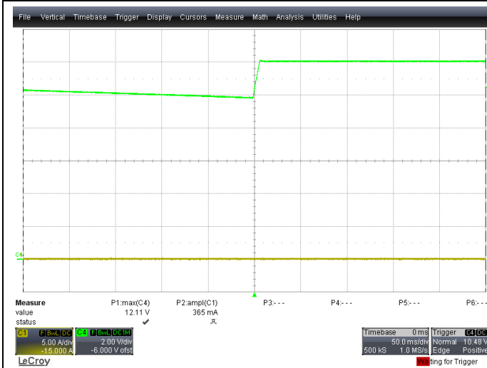
Figure 13 - Softstart from precharge at no load (zoom in) Green trace: Output voltage, 2V/div, 50ms/div Blue trace: Load current, 10A/div, 50ms/div
