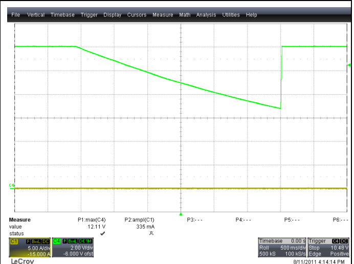
Figure 14 - Softstart from precharge at no load (zoom out) Green trace: Output voltage, 2V/div, 500ms/div Blue trace: Load current, 10A/div, 500ms/div
