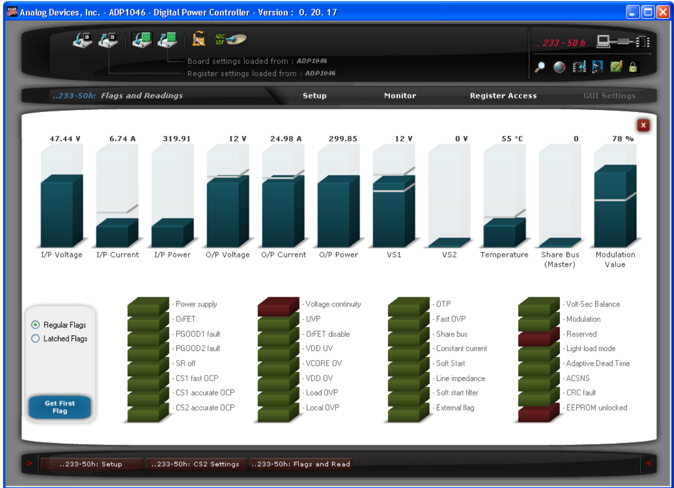
Figure 7 - Monitor window in GUI showing entire status of the PSU
