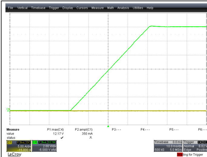
Figure 11 - Startup at 42VDC, no load Green trace: Output voltage, 2V/div, 10ms/div Yellow trace: Load current, 5A/div, 10ms/div
