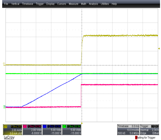
Figure 60 – Output reverse current protection, OrFET enable threshold 0mV Red trace: OrFET gate signal Green and Blue trace: Output voltages of two power supplies Yellow trace: Load current of power supply that is softstarting
