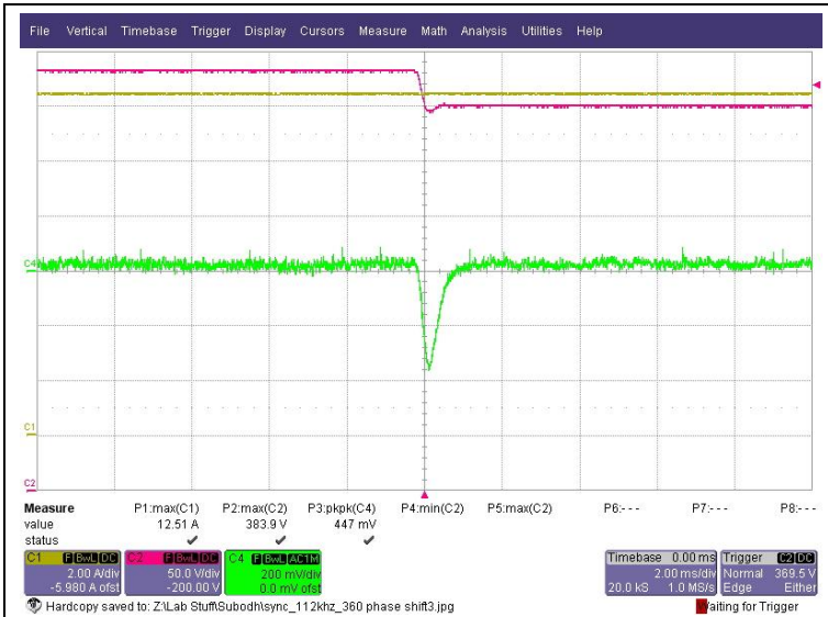
Figure 42 – Line voltage Feed forward DISABLED, 600W load Red trace: Input voltage step 350-385VDC, 50V/div Green trace: Output voltage (AC Coupled), 200mV/div
