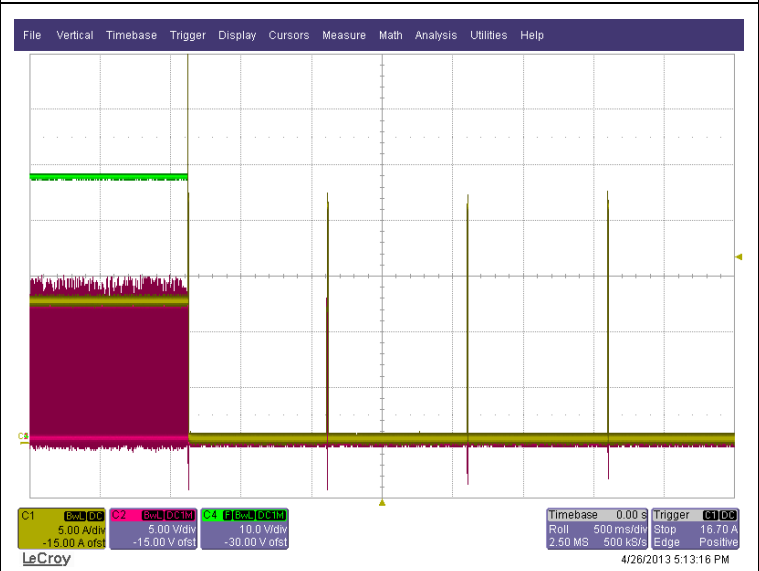
Figure 19 - Over current protection, HICCUP MODE, 385VDC, 600W to output shorted Red trace: SR drive, 5V/div, 5ms/div Green trace: Output voltage 10V/div, 200us/div Yellow trace: Output current 5A/div
