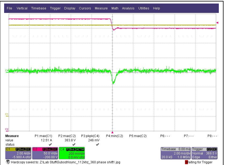
Figure 43 – Line voltage Feed forward ENABLED, 600W load Red trace: Input voltage step 350-385VDC, 50V/div Green trace: Output voltage (AC Coupled), 200mV/div
