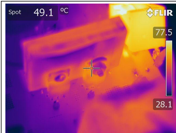
Figure 68 – Thermals, Primary MOSFET
