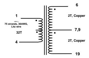
Figure 23 - Transformer electrical diagram
