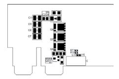
Figure 37 – Bottom side placement of components
