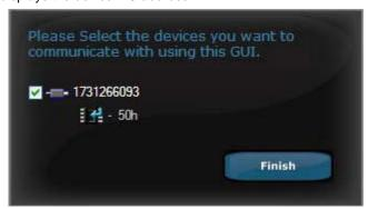
Figure 4 - ADP1046A address of 50h in the GUI
