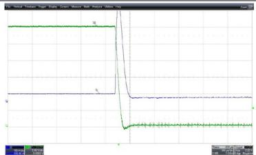
Figure 13 –Over current protection, 600Wto output shorted, Green trace: Output voltage, 2V/div, 500us/div Blue trace: Load current, 100A/div, 500us/div
