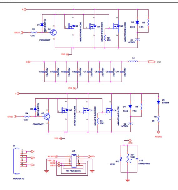
Figure 28 – Schematic – SR & Thermal sense
