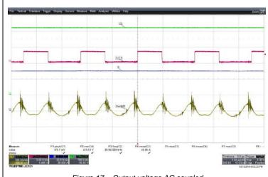
Figure 17 - Output voltage AC coupled 400VDC, 50A, 100mV/div, 5us/div..
