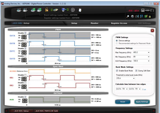
Figure 9 – PWM Settings window in the GUI
