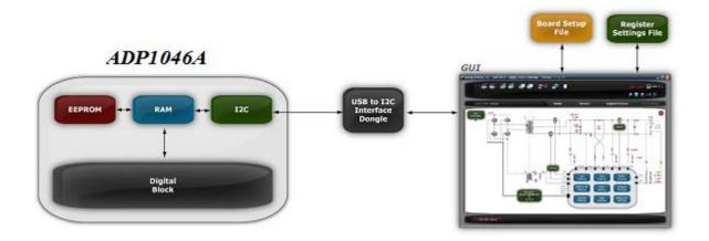
Figure 3 - ADP1046A and GUI interaction
