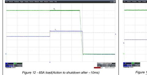
Figure 12 - 65A load(Action to shutdown after ~10ms) Green trace: Output voltage, 2V/div, 5ms/div Blue trace: Load current, 20A/div, 5ms/div
