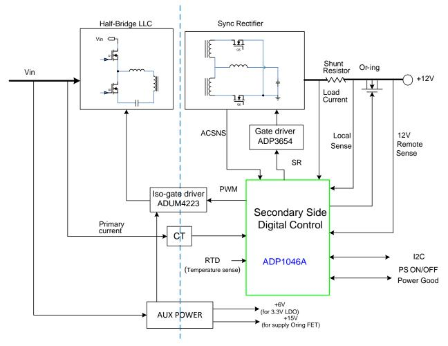
Figure.2 – The LLC EVB Block Diagram
