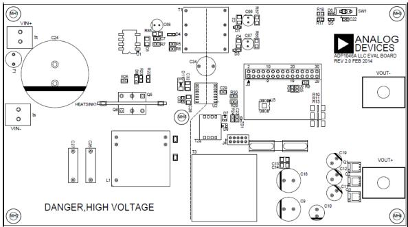
Figure 30 – Top side placement of components
