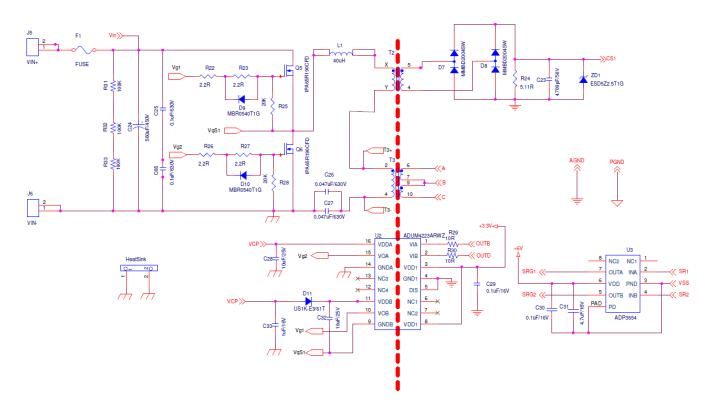
Figure 25 – Schematic – Half Bridge LLC
