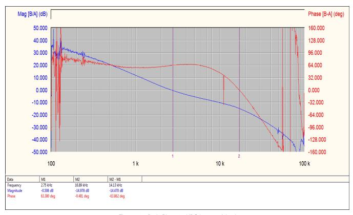
Figure 21 – Bode Plots, 400VDC input, 50A load, Blue trace: Gain in dB Red trace: Phase in degrees Crossover frequency= 2.75KHz Phase margin= 63.38°
