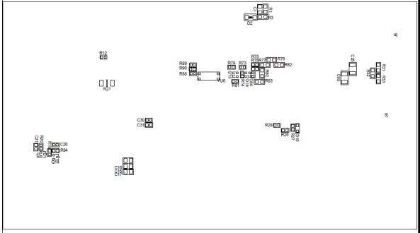
Figure 2 – Bottom side placement of components
