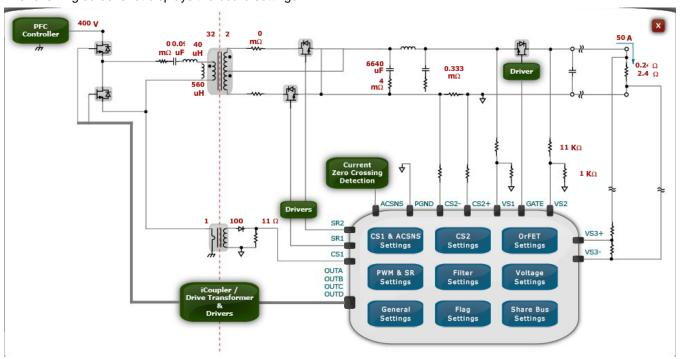
Figure 7 - Main Setup window of ADP1046A GUI
