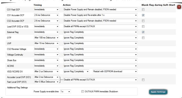
Figure 8 - Fault Configurations
