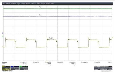
Figure 16 – Synchronous rectifier MOSFET Peak reverse voltage at 600W load, 400VDC, 50V/div, 2us/div
