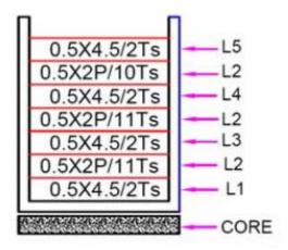
Figure 24 - Transformer construction diagram
