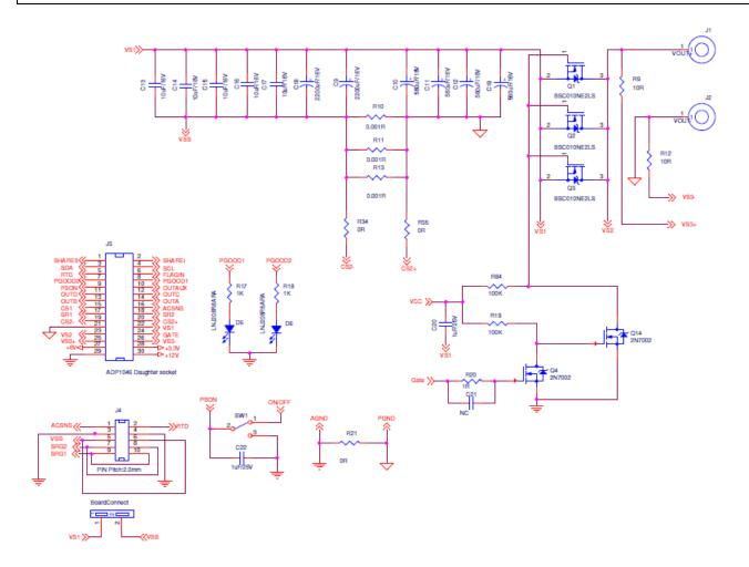
Figure 26 – Schematic – Current sense & Oring FET
