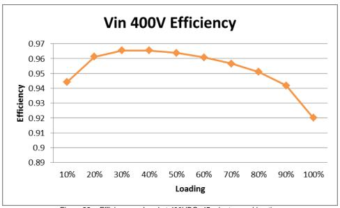
Figure 22 - Efficiency vs Load at 400VDC, 45 minutes soaking time
