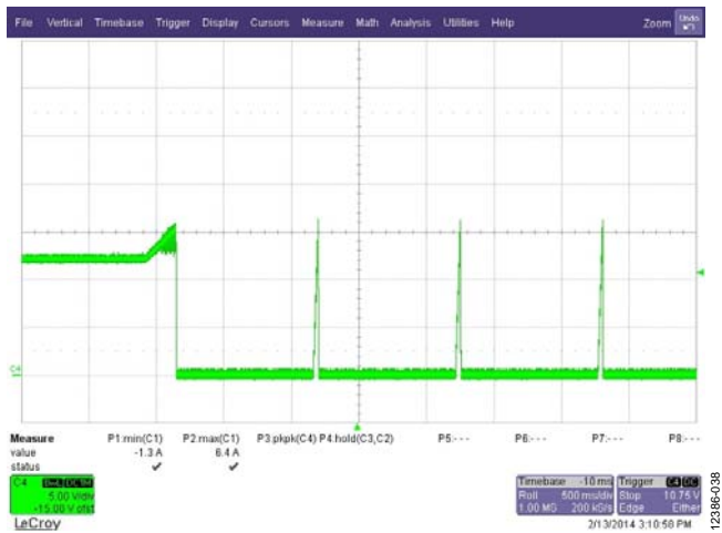
Figure 38. VOUT_OV_FAST_FAULT Fault Response Set to Shut Down and Retry Indefinitely Green Trace: Output Voltage
