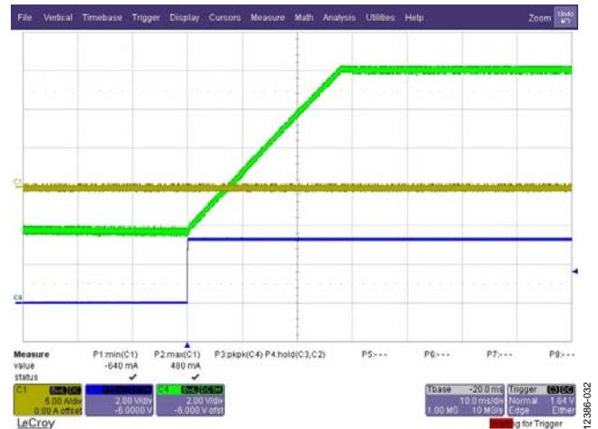
Figure 32. PSU Soft Start from Precharge Green Trace: Output Voltage Blue Trace: Hardware PS_ON Yellow Trace: Primary Current
