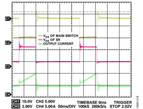
Figure 17. MOSFET Drain to Source Voltages at 60 Vdc Input and 3 A Load
