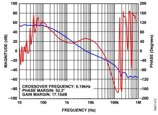
Figure 12. Loop Gain Measurement
