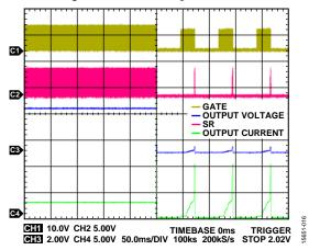
Figure 15. OCP Under Output Short Circuit at 48 Vdc and 3 A Load
