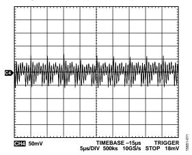
Figure 11. Output Ripple at 48 Vdc Input, 3 A load
