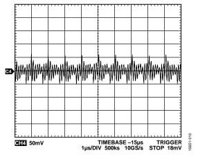
Figure 10. Output Ripple at 48 Vdc Input, No Load
