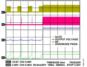
Figure 16. Recovery from Output Short Circuit at 48 Vdc and 3 A Load
