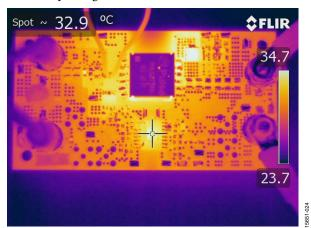
Figure 22. Thermal Image at 48 Vdc Input, 3 A Load, No Airflow, 0.5 Hour Soaking Time
