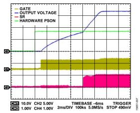
Figure 7. Soft Start at 48 Vdc Input, No Load
