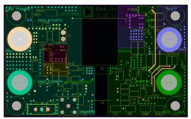
Figure 28. PCB Layout, Layer 3
