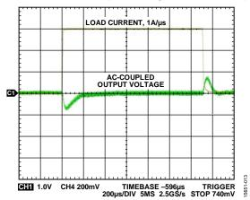
Figure 13. Transient Response with Load Steps: 0% to 100%
