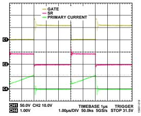
Figure 18. Peak Primary Current at 36 Vdc Input and 3 A Load
