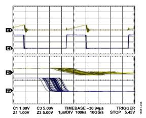
Figure 6. GATE Falling Edge Jitter at 48 Vdc Input and 3 A Load
