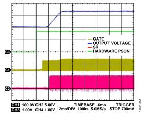
Figure 8. Soft Start from Precharge
