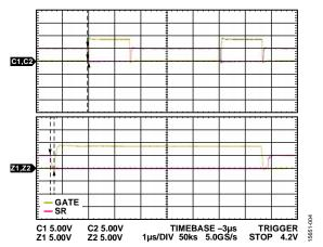
Figure 4. Deadtime Example at 48 Vdc Input and No Load
