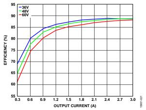
Figure 19. Efficiency Curves at 36 Vdc, 48 Vdc, 60 Vdc Input
