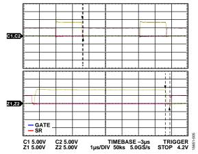
Figure 5. Deadtime Example at 48 Vdc Input and No Load
