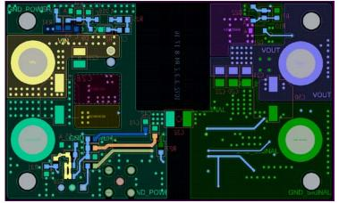
Figure 29. PCB Layout, Layer 4
