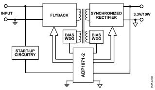
Figure 2. ADP1071-2EBZ3.3V Evaluation Board Block Diagram
