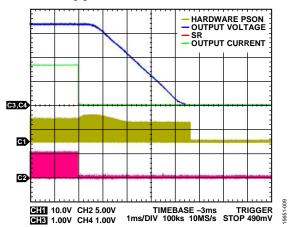
Figure 9. Soft Stop at 48 Vdc Input, 3 A Load
