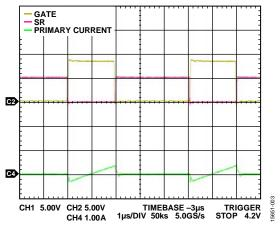
Figure 3. GATE and SR Example at 48 Vdc Input and No Load
