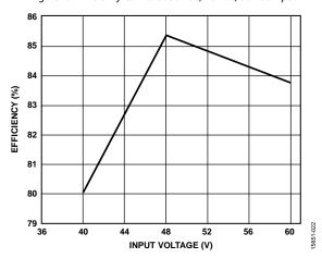
Figure 20. Efficiency vs. Input Voltage
