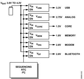
Figure 2. Typical Power Domains in a Portable System
