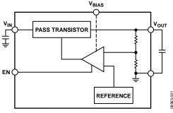
Figure 1. An LDO Regulates the Output Voltage with a Low Dropout Voltage (The Difference Between  $V_{OUT}$  and the Lowest Specified Value of  $V_{IN}$  at the Rated Load Current)
