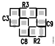
Figure 2. Loop Filter Layout
