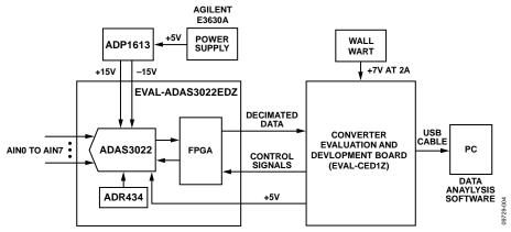
Figure 4. Test Setup Functional Block Diagram
