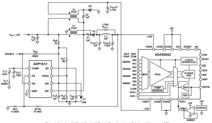
Figure 1. Complete 5 V, Single-Supply, 8-Channel Data Acquisition Solution with Integrated PGIA (Simplified Schematic: All Connections and Decoupling Not Shown)
