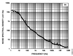
Figure 16. NSD vs. Frequency at  $V_{IN}$  = 1.8 V,  $I_0$  = 5 A NSD of Active Paralleling
