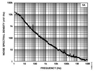
Figure 15. Noise Spectral Density (NSD) vs. Frequency at  $V_{IN} = 1.8 V$ ,  $I_0 = 5 A$ NSD of Passive Paralleling
