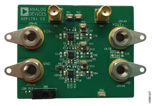
Figure 7. Passive Current Sharing Evaluation Board
