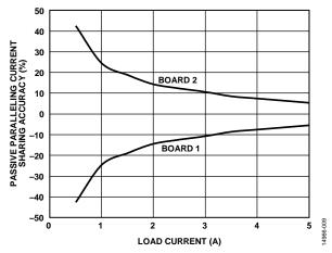
Figure 9. Passive Paralleling Current Sharing Accuracy vs. Load Current
