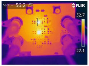
Figure 17. Thermal Test of Passive Paralleling
