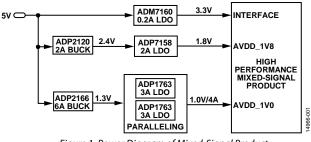
Figure 1. Power Diagram of Mixed-Signal Product
