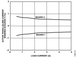
Figure 10. Active Paralleling Current Sharing Accuracy vs. Load Current
