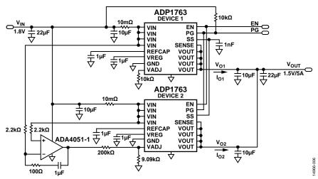
Figure 6. Active Paralleling the Two ADP1763 Devices
