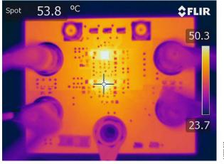
Figure 18. Thermal Test of Active Paralleling
