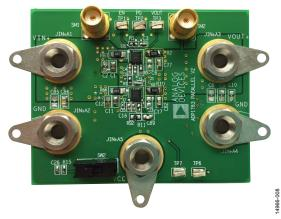
Figure 8. Active Current Sharing Evaulation Board
