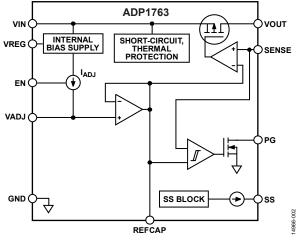
Figure 2. ADP1763 Internal Block Diagram
