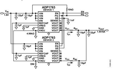
Figure 3. Passive Paralleling the Two ADP1763 Devices
