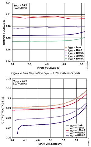
Figure 5. Line Regulation,  $V_{OUT} = 3.3 V$ , Different Loads
