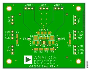
Figure 8. PCB Layout, Top
