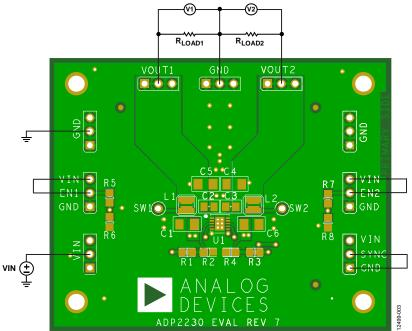
Figure 3. Output Voltage Measurement Setup
