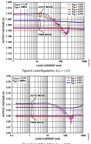
Figure 7. Load Regulation, Vout = 3.3 V
