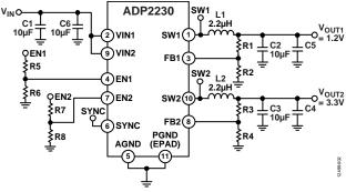
Figure 2. ADP2230 Evaluation Board Schematic
