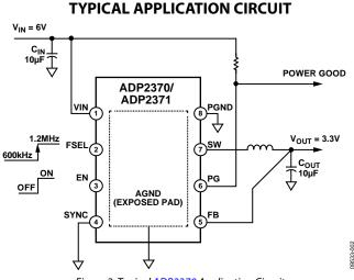
Figure 2. Typical ADP2370 Application Circuit
