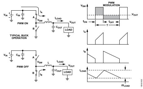
Figure 3. Buck Mode When VIN > VOUT
