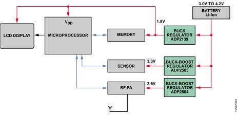
Figure 1. Typical Low Power Portable System
