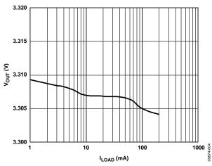
Figure 4. Output Voltage vs. Load Current,  $V_{RIPPLE} = 50 \text{ mV}$ ,  $C_{OUT} = 1 \mu F$
