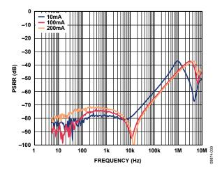
Figure 32. Power Supply Rejection Ratio vs. Frequency,  $V_{OUT} = 1.5 V$ ,  $V_{IN} = 2.5 V$ ,  $V_{RIPPLE} = 50 \text{ mV}$ ,  $C_{OUT} = 1 \mu F$
