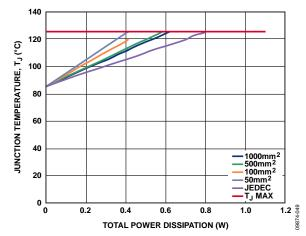
Figure 55. Junction Temperature vs. Total Power Dissipation,  $T_A = 85^{\circ}C$
