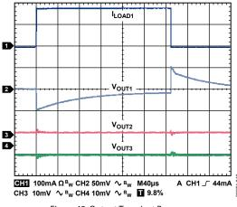
Figure 48. Output Transient Response,  $I_{LOAD1} = 1 \text{ mA to } 200 \text{ mA}, I_{LOAD2} = 1 \text{ mA}, I_{LOAD3} = 1 \text{ mA},$  $CH1 = I_{LOAD1}, CH2 = V_{OUT1}, CH3 = V_{OUT2}, CH4 = V_{OUT3}$
