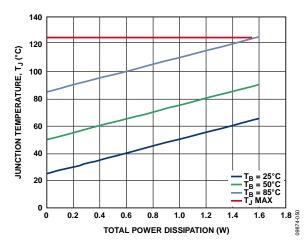
Figure 56. Junction Temperature vs. Total Power Dissipation and Board Temperature
