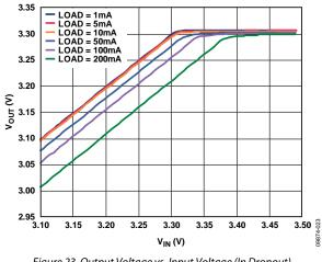
Figure 23. Output Voltage vs. Input Voltage (In Dropout),  $V_{OUT1} = 3.3 V$ ,  $V_{RIPPLE} = 50 mV$ ,  $C_{OUT} = 1 \mu F$
