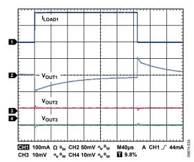
Figure 40. Load Transient Response,  $I_{LOAD1} = 1 \text{ mA to } 200 \text{ mA}, I_{LOAD2} = I_{LOAD3} = 1 \text{ mA}, CH1 = I_{LOAD1},$  $CH2 = V_{OUT1}, CH3 = V_{OUT2}, CH4 = V_{OUT3}, V_{RIPPLE} = 50 \text{ mV}, C_{OUT} = 1 \mu F$
