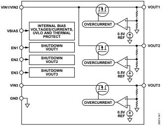
Figure 47. Internal Block Diagram
