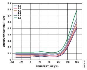
Figure 21. Shutdown Current vs. Temperature at Various Input Voltages,  $V_{\text{RIPPLE}} = 50$  mV,  $C_{\text{OUT}} = 1 \, \mu\text{F}$
