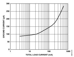
Figure 16. Ground Current vs. Load Current, All Outputs Loaded Equally,  $V_{\text{RIPPLE}} = 50 \text{ mV}, C_{\text{OUT}} = 1 \, \mu F$
