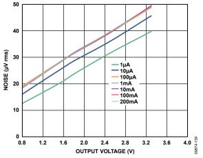
Figure 39. Output Noise vs. Output Voltage, Different Load Currents,  $V_{IN} = 5 V$ ,  $V_{RIPPLE} = 50 \text{ mV}$ ,  $C_{OUT} = 1 \mu F$
