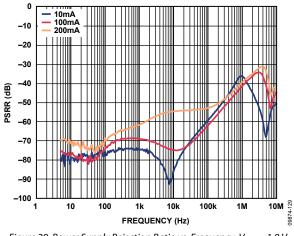
Figure 29. Power Supply Rejection Ratio vs. Frequency,  $V_{OUT} = 1.8$  V,  $V_{IN} = 2.3$  V,  $V_{RIPPLE} = 50$  mV,  $C_{OUT} = 1$   $\mu$ F
