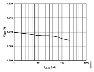
Figure 7. Output Voltage vs. Load Current,  $V_{RIPPLE} = 50 \text{ mV}$ ,  $C_{OUT} = 1 \mu F$
