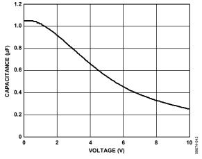
Figure 49. Capacitance vs. Voltage Bias Characteristic
