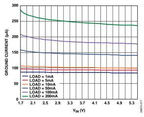
Figure 17. Ground Current vs. Input Voltage, All Outputs Loaded Equally,  $V_{\text{RIPPLE}} = 50$  mV,  $C_{\text{OUT}} = 1 \, \mu\text{F}$
