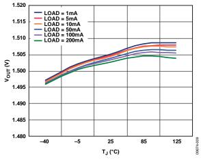
Figure 9. Output Voltage vs. Junction Temperature,  $V_{RIPPLE} = 50 \text{ mV}$ ,  $C_{OUT} = 1 \mu F$
