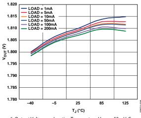
Figure 6. Output Voltage vs. Junction Temperature,  $V_{RIPPLE} = 50 \text{ mV}$ ,  $C_{OUT} = 1 \mu F$
