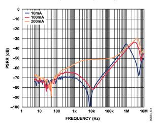
Figure 31. Power Supply Rejection Ratio vs. Frequency,  $V_{OUT} = 3.3 V$ ,  $V_{IN} = 3.8 V$ ,  $V_{RIPPLE} = 50 \text{ mV}$ ,  $C_{OUT} = 1 \mu F$
