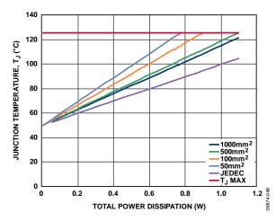
Figure 54. Junction Temperature vs. Total Power Dissipation,  $T_A = 50^{\circ}C$
