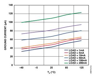
Figure 12. Ground Current vs. Junction Temperature, Single Output Loaded,  $V_{\text{RIPPLE}} = 50 \text{ mV}$ ,  $C_{\text{OUT}} = 1 \, \mu F$
