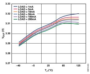
Figure 3. Output Voltage vs. Junction Temperature,  $V_{RIPPLE} = 50 \text{ mV}$ ,  $C_{OUT} = 1 \mu F$
