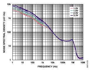
Figure 36. Output Noise Spectral Density,  $V_{IN} = 5 V$ ,  $I_{LOAD} = 10 mA$ ,  $V_{RIPPLE} = 50 mV$ ,  $C_{OUT} = 1 \mu F$
