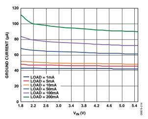
Figure 14. Ground Current vs. Input Voltage, Single Output Loaded,  $V_{\text{RIPPLE}} = 50 \text{ mV}, C_{\text{OUT}} = 1 \, \mu F$
