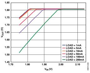
Figure 26. Output Voltage vs. Input Voltage (in Dropout),  $V_{OUT2} = 1.8 V$ ,  $V_{RIPPLE} = 50 mV$ ,  $C_{OUT} = 1 \mu F$
