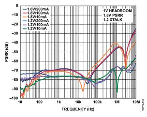
Figure 35. Power Supply Rejection Ratio vs. Frequency, Channel to Channel Crosstalk,  $V_{RIPPLE} = 50 \text{ mV}$ ,  $C_{OUT} = 1 \mu F$
