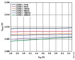
Figure 5. Output Voltage vs. Input Voltage,  $V_{RIPPLE} = 50 \text{ mV}$ ,  $C_{OUT} = 1 \mu F$
