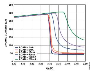
Figure 24. Ground Current vs. Input Voltage (in Dropout),  $V_{OUT1} = 3.3 V$ ,  $V_{RIPPLE} = 50 \text{ mV}$ ,  $C_{OUT} = 1 \mu F$
