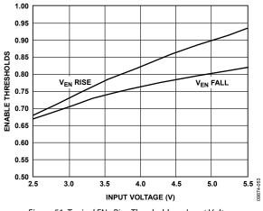
Figure 51. Typical ENx Pins Thresholds vs. Input Voltage
