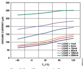
Figure 15. Ground Current vs. Junction Temperature, All Outputs Loaded Equally,  $V_{RIPPLE} = 50 \text{ mV}$ ,  $C_{OUT} = 1 \mu F$
