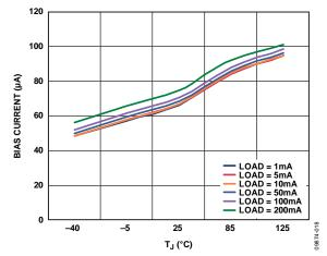
Figure 18. Bias Current vs. Junction Temperature, Single Output Loaded,  $V_{RIPPLE} = 50 \text{ mV}, C_{OUT} = 1 \mu F$
