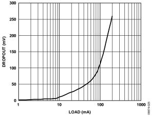
Figure 25. Dropout Voltage vs. Load Current and Output Voltage,  $V_{OUT2} = 1.8$  V,  $V_{RIPPLE} = 50$  mV,  $C_{OUT} = 1$   $\mu$ F
