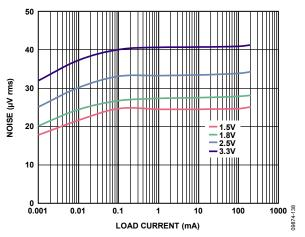
Figure 38. 100 Hz to 100 kHz Output Noise vs. Load Current and Output Voltage,  $V_{IN} = 5 V$ ,  $V_{RIPPLE} = 50 mV$ ,  $C_{OUT} = 1 \mu F$
