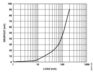
Figure 22. Dropout Voltage vs. Load Current and Output Voltage,  $V_{OUT1} = 3.3 V$ ,  $V_{RIPPLE} = 50 mV$ ,  $C_{OUT} = 1 \, \mu F$
