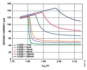
Figure 27. Ground Current vs. Input Voltage in Dropout),  $V_{OUT2} = 1.8 V$ ,  $V_{RIPPLE} = 50 mV$ ,  $C_{OUT} = 1 \mu F$
