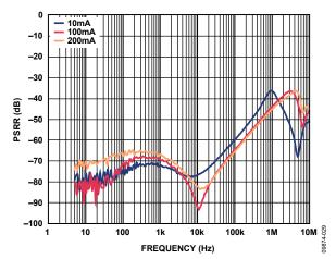
Figure 30. Power Supply Rejection Ratio vs. Frequency,  $V_{OUT} = 3.3 V$ ,  $V_{IN} = 4.3 V$ ,  $V_{RIPPLE} = 50 \text{ mV}$ ,  $C_{OUT} = 1 \mu F$
