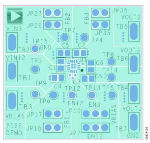
Figure 57. Example of PCB Layout, Top Side
