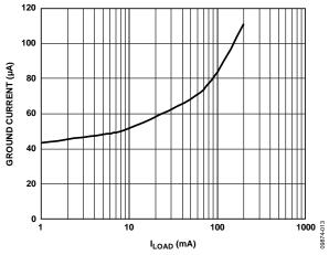
Figure 13. Ground Current vs. Load Current, Single Output Loaded,  $V_{\text{RIPPLE}} = 50 \text{ mV}, C_{\text{OUT}} = 1 \, \mu F$
