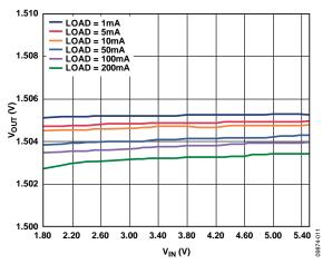
Figure 11. Output Voltage vs. Input Voltage,  $V_{RIPPLE} = 50 \text{ mV}$ ,  $C_{OUT} = 1 \mu F$
