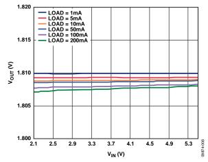
Figure 8. Output Voltage vs. Input Voltage,  $V_{RIPPLE} = 50 \text{ mV}$ ,  $C_{OUT} = 1 \mu F$
