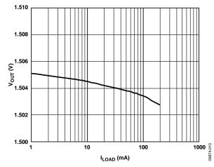
Figure 10. Output Voltage vs. Load Current,  $V_{RIPPLE} = 50 \text{ mV}$ ,  $C_{OUT} = 1 \mu F$
