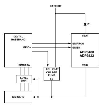
Figure 3. Blocking Diode on BAT Input
