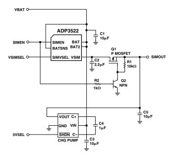
Figure 5. Load Switch Circuit
