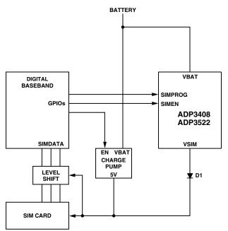
Figure 2. Blocking Diode on SIM Output
