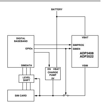
Figure 4. Load Switch on SIM Output
