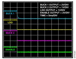
Figure 21. Three Regulators Turned Off by Sequencer
