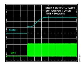
Figure 17. Buck 1 Enable Startup
