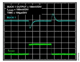
Figure 10. Buck 1 Load Transient Response
