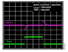
Figure 13. Buck 2 Load Transient Response
