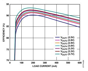
Figure 9. Buck 1, Efficiency vs. Load Current
