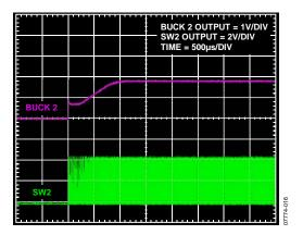
Figure 16. Buck 2 Enable Startup
