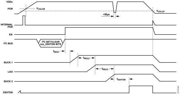
Figure 25. Activation and Power Failure Conditions
