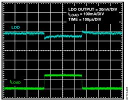
Figure 7. LDO Load Transient
