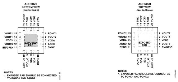
*Figure 4. Pin Configuration (Bottom View)*
