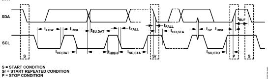
Figure 3. I<sup>2</sup>C Interface Timing Diagram
