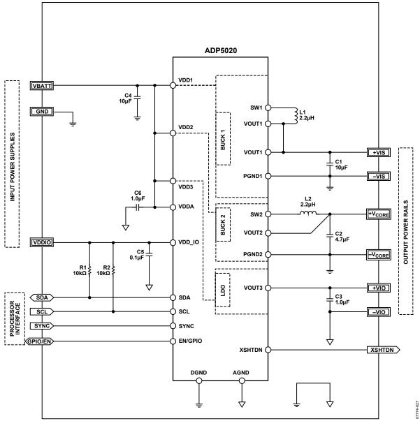
Figure 29. Schematic for Camera Module Applications
