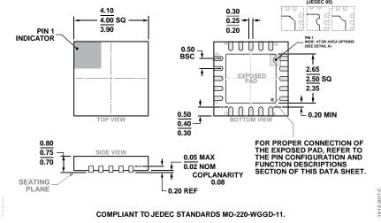
Figure 30. 20-Lead Lead Frame Chip Scale Package [LFCSP] 4 mm × 4 mm Body and 0.75 mm Package Height (CP-20-10) Dimensions shown in millimeters
