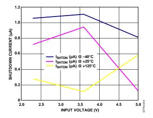
Figure 14. Shutdown Current vs. Input Voltage
