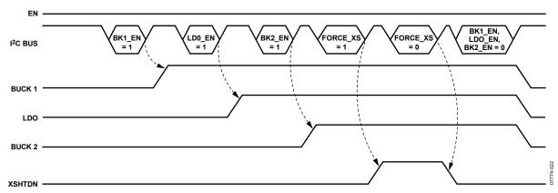
Figure 26. Individual Activation Through I<sup>2</sup>C Commands
