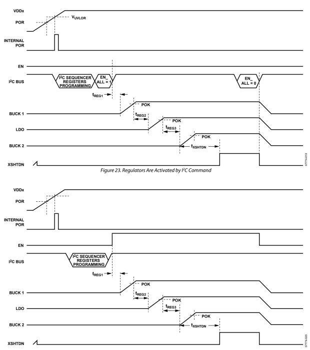
Figure 24. Activation Command Using the EN Pin
