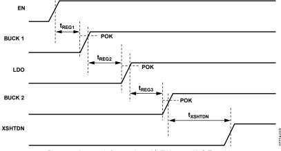
Figure 22. Automatic Sequencing with EN Low-to-High Transition
