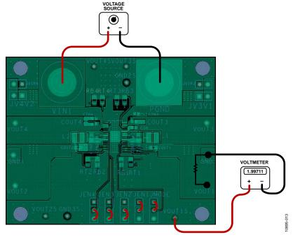
Figure 16. Output Voltage Measurement
