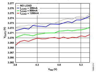
Figure 9. Buck Regulator Line Regulation,  $V_{OUT2} = 3.3 \text{ V}$
