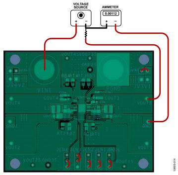
Figure 17. Ground Current Measurement
