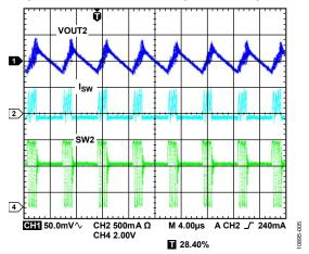
Figure 5. Typical Waveforms,  $V_{OUT2} = 3.3 \text{ V}$ ,  $I_{OUT2} = 30 \text{ mA}$ , PSM Mode
