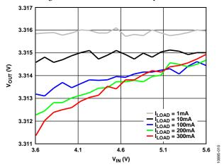
Figure 13. V<sub>OUT</sub> vs. V<sub>IN</sub>, LDO Line Regulation for an Output of 3.3 V
