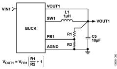
Figure 2. BUCK1 External Output Voltage Setting
