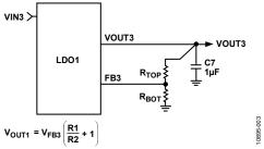
Figure 3. LDO1 External Output Voltage Setting
