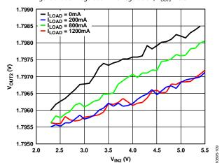
Figure 10. Buck Regulator Line Regulation,  $V_{OUT2} = 1.8 \text{ V}$
