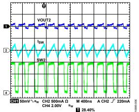
Figure 6. Typical Waveforms,  $V_{OUT2} = 3.3 \text{ V}$ ,  $I_{OUT2} = 30 \text{ mA}$ , PWM Mode
