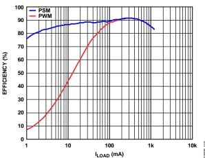
Figure 12. Buck Regulator Efficiency,  $V_{IN2} = 3.6 \text{ V}$ ,  $V_{OUT2} = 1.8 \text{ V}$
