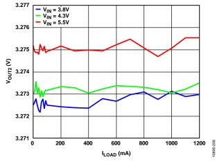
Figure 7. Buck Load Regulation,  $V_{OUT2} = 3.3 \text{ V}$
