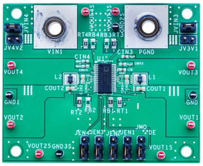
Figure 19. Evaluation Board of the ADP5034 TSSOP
