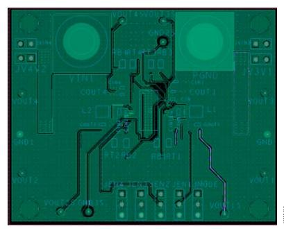
Figure 21. Bottom Layer, Recommended Layout for ADP5034 TSSOP
