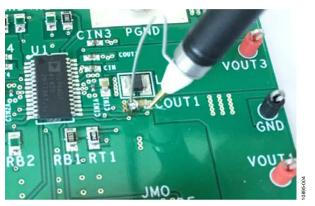
Figure 4. Measuring Output Voltage Ripple
