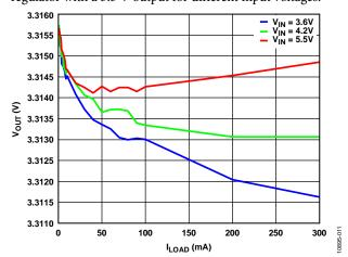
Figure 14. V<sub>OUT</sub> vs. I<sub>LOAD</sub>, LDO Load Regulation
