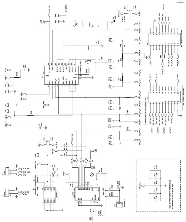
Figure 7. ADP5062 LFCSP Demo Board Schematic
