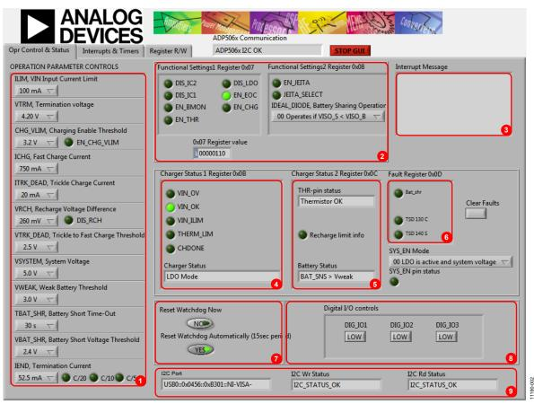
Figure 2. ADP5062 GUI Operation Control and Status Tab
