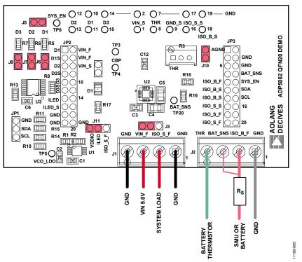
Figure 5. ADP5062CP-EVALZ Typical Operation Setup
