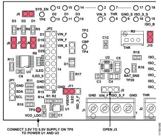
Figure 6. Board Setup for VINx Input Quiescent Current Measurement
