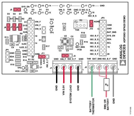
Figure 5. ADP5063 LFCSP Demo Board Typical Operation Setup
