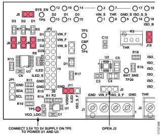
Figure 6. Board Setup for VINx Quiescent Current Measurement
