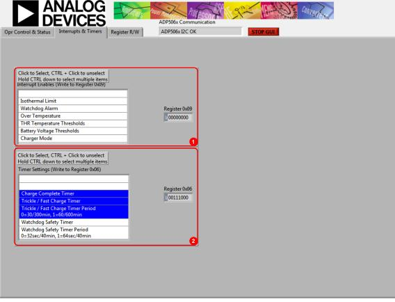
Figure 3. ADP5063 Evaluation Software GUI, Interrupts & Timers Tab
