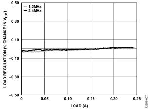
Figure 9. Boost Regulator Load Regulation,  $V_{IN} = 5 V$ ,  $V_{POS} = 15 V$  (Nominal Defined as Average Value Within a Range of 65% to 75% Maximum Load)
