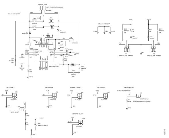
Figure 13. Evaluation Board Schematic for the ADP5070/ADP5071
