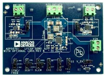
Figure 1. ADP5070CP-EVALZ/ADP5071CP-EVALZ LFCSP Evaluation Board
