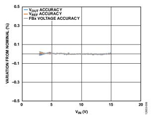
Figure 8. Inverting Regulator Line Regulation,  $V_{NEG} = -15$  V,  $f_{SW} = 1.2$  MHz, 15 mA Load,  $T_A = 25$ °C (Nominal Defined as Average Value Within a Range of 10% to 90%  $V_{NV}$ )
