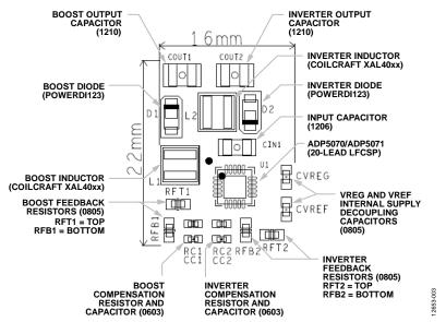
Figure 3. ADP5070/ADP5071 Top Component Detail
