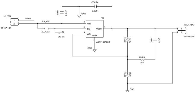
Figure 14. Evaluation Board Schematic for the Optional LDO Regulators (LFCSP Package Version)
