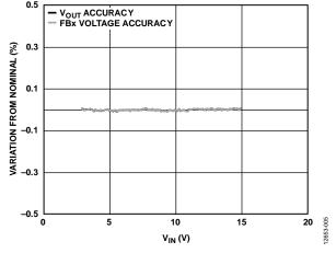
Figure 7. Boost Regulator Line Regulation,  $V_{POS} = 15 \text{ V}$ ,  $f_{SW} = 1.2 \text{ MHz}$ , 15 mA Load,  $T_A = 25^{\circ}\text{C}$  (Nominal Defined as Average Value Within a Range of 10% to 90%  $V_{\text{IV}}$ )
