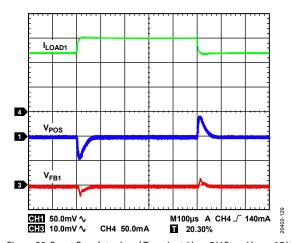
Figure 29. Boost Regulator Load Transient,  $V_{IN} = 5$  V Step,  $V_{POS} = 15$  V,  $I_{LOAD1} = 120$  mA to 150 mA Step,  $f_{SW} = 2.4$  MHz,  $T_A = 25$ °C
