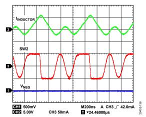
Figure 37. Inverting Regulator Discontinuous Conduction Mode Operation Showing  $I_{INDUCTOR}$ , Switch Node Voltage, and Output Ripple,  $V_{IN} = +5 V$ ,  $V_{NEG} = -5 V$ ,  $I_{LOAD2} = 6 \text{ mA}$ ,  $f_{SW} = 2.4 \text{ MHz}$ ,  $T_A = 25^{\circ}\text{C}$
