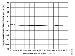
Figure 21. Cross Regulation, Boost Regulator  $V_{FB1}$  Regulation over Inverting Regulator Current Load,  $V_{IN}=+5$  V,  $V_{POS}=+15$  V,  $V_{NEG}=-15$  V,  $f_{SW}=2.4$  MHz,  $T_A=25$ °C, Boost Regulator Run in Continuous Conduction Mode with Fixed Load for Test
