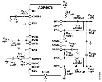
Figure 46. Typical +5 V to  $\pm 15$  V Application
