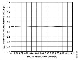
Figure 24. Cross Regulation, Inverting Regulator  $V_{FB2}$  Regulation over Boost Regulator Current Load,  $V_{IN} = +5 V$ ,  $V_{POS} = +15 V$ ,  $V_{NEG} = -15 V$ ,  $f_{SW} = 2.4$  MHz,  $T_A = 25$ °C, Inverting Regulator Run in Continuous Conduction Mode with Fixed Load for Test
