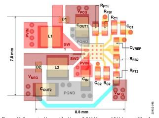
Figure 48. Suggested Layout for  $V_{IN} = +3.3 V$ ,  $V_{POS} = +15 V$ ,  $I_{LOAD1} = 90$  mA and  $V_{NEG} = -15 V$ ,  $I_{LOAD2} = 60$  mA, Not to Scale
