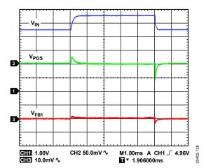
Figure 28. Boost Regulator Line Transient,  $V_N$  = 4.5 V to 5.5 V Step,  $V_{POS}$  = 15 V, Resistor Load for Boost Regulator ( $R_{LOAD1}$ ) = 300  $\Omega$ ,  $f_{SW}$  = 2.4 MHz,  $T_A$  = 25 °C
