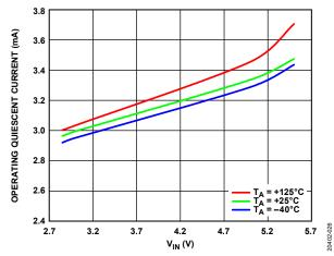
Figure 30. Operating Quiescent Current vs. V<sub>IN</sub> over Temperature, ENx Pins On
