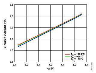
Figure 27. Standby Current vs. V<sub>IN</sub> over Temperature, ENx Pins Below Shutdown Threshold
