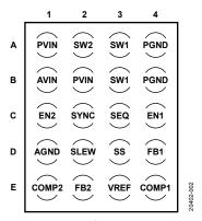
Figure 2. Pin Configuration (Top View)
