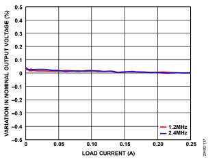
Figure 17. Boost Regulator Load Regulation,  $V_{IN} = 5 V$ ,  $V_{POS} = 15 V$
