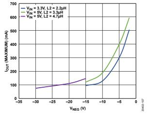
Figure 7. Inverting Regulator Maximum Output Current,  $f_{SW} = 2.4$  MHz,  $T_A = 25$ °C, Based on Target of 70%  $I_{LIM}$  (INVERTER)
