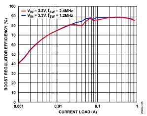
Figure 5. Boost Regulator Efficiency vs. Current Load,  $V_{IN}=3.3~V, V_{POS}=5~V, T_A=25^{\circ}\text{C}$
