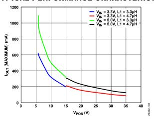
Figure 3. Boost Regulator Maximum Output Current,  $f_{SW} = 1.2$  MHz,  $T_A = 25$ °C, Based on Target of 70%  $I_{LIM (BOOST)}$
