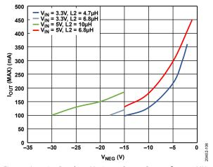
Figure 6. Inverting Regulator Maximum Output Current,  $f_{SW} = 1.2$  MHz,  $T_A = 25$ °C, Based on Target of 70%  $I_{LIM}$  (INVERTER)
