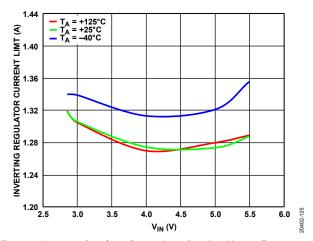
Figure 25. Inverting Regulator Current Limit ( $I_{LIMIT2}$ ) vs.  $V_{IN}$  over Temperature
