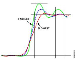
Figure 40. Switching Node at Various Slew Rate Settings
