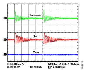
Figure 33. Boost Regulator Skip Mode Operation Showing Inductor Current ( $I_{INDUCTOR}$ ), Switch Node Voltage, and Output Ripple,  $V_{IN} = 5 \text{ V}$ ,  $V_{POS} = 15 \text{ V}$ ,  $I_{LOADI} = 4 \text{ mA}$ ,  $f_{SW} = 2.4 \text{ MHz}$ ,  $T_A = 25 ^{\circ}\text{C}$
