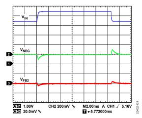
Figure 31. Inverting Regulator Line Transient,  $V_{\text{IN}} = +4.5 \text{ V}$  to +5.5 V Step,  $V_{\text{NEG}} = -15 \text{ V}$ , Resistor Load for Inverting Regulator ( $R_{\text{LOAD2}}$ ) =  $300 \Omega$ ,  $f_{\text{SW}} = 2.4 \text{ MHz}$ ,  $T_{\text{A}} = 25 ^{\circ}\text{C}$
