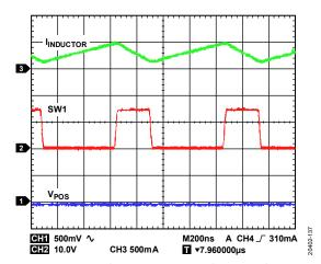
Figure 35. Boost Regulator Continuous Conduction Mode Operation Showing  $I_{INDUCTOR}$ , Switch Node Voltage, and Output Ripple,  $V_{IN} = 5 V$ ,  $V_{POS} = 15 V$ ,  $I_{LOAD1} = 90 \text{ mA}$ ,  $f_{SW} = 2.4 \text{ MHz}$ ,  $T_A = 25 ^{\circ}\text{C}$
