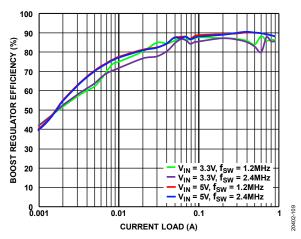
Figure 9. Boost Regulator Efficiency vs. Current Load,  $V_{POS} = 9 V$ ,  $T_A = 25$ °C
