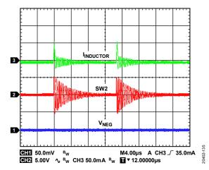
Figure 36. Inverting Regulator Skip Mode Operation Showing  $I_{INDUCTOR}$ , Switch Node Voltage, and Output Ripple,  $V_{IN} = +5 V$ ,  $V_{NEG} = -5 V$ ,  $I_{LOAD2} = 0 \text{ mA}$ ,  $f_{SW} = 2.4 \text{ MHz}$ ,  $T_A = 25^{\circ}\text{C}$
