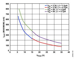
Figure 4. Boost Regulator Maximum Output Current,  $f_{SW} = 2.4$  MHz,  $T_A = 25$ °C, Based on Target of 70%  $I_{LIM(BOOST)}$
