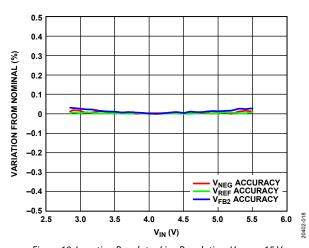
Figure 19. Inverting Regulator Line Regulation,  $V_{NEG} = -15 V$ ,  $f_{SW} = 1.2$  MHz, 15 mA Load,  $T_A = 25$  °C
