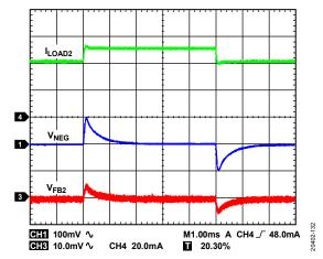
Figure 32. Inverting Regulator Load Transient,  $V_{IN} = +5$  V Step,  $V_{NEG} = -15$  V,  $I_{LOAD2} = 35$  mA to 45 mA Step,  $f_{SW} = 2.4$  MHz,  $T_A = 25$ °C
