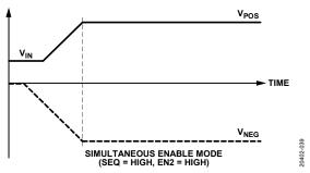
Figure 41. Simultaneous Enable Mode
