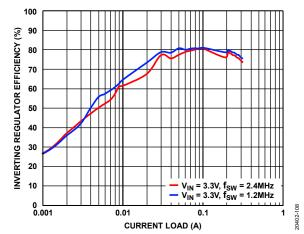
Figure 8. Inverting Regulator Efficiency vs. Current Load,  $V_{IN} = +3.3 V$ ,  $V_{NEG} = -5 V$ ,  $T_A = 25 ^{\circ} C$
