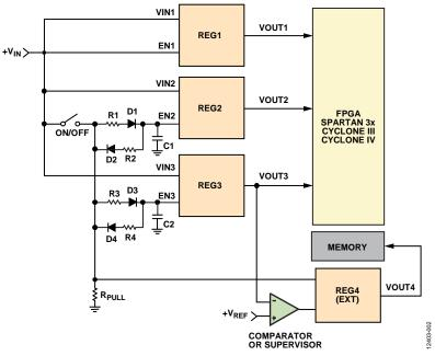
Figure 2. Simple Power Supply Sequencing Method Using Resistors, Capacitors, and Diodes
