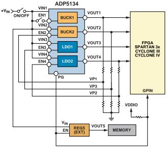
Figure 5. Simple Sequencing with the ADP5134
