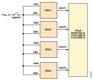
Figure 1. Typical Method for Powering Processors and FPGAs
