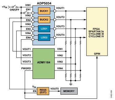
Figure 8. Sequencing the ADP5034 4-Channel Regulator Using the ADM1184 Quad Voltage Monitor
