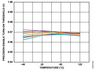
Figure 3. Precision Enable Turn-On Threshold over Temperature, 10 Samples
