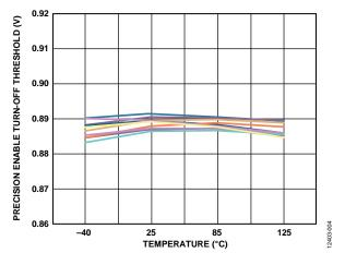
Figure 4. Precision Enable Turn-Off Threshold over Temperature, 10 Samples
