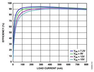
Figure 14. Channel 1 PWM Efficiency vs. Load Current,  $V_{OUT1} = 5 V$
