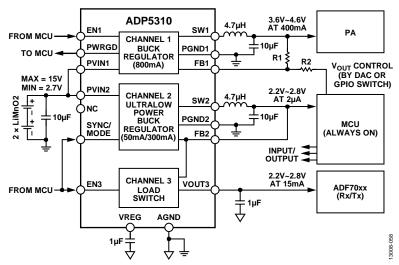
Figure 58. Typical Application of a Smart Meter
