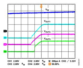
Figure 41. Soft Start Waveform
