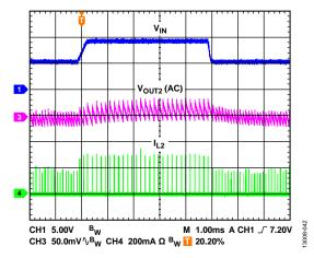
Figure 42. Channel 2 Line Transient in Hysteresis Mode
