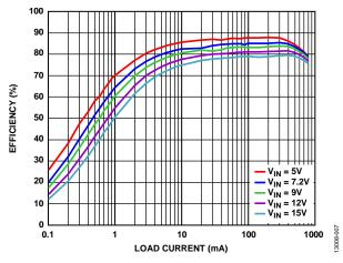
Figure 7. Channel 1 Auto PSM/PWM Efficiency vs. Load Current, V<sub>OUT1</sub> = 1.8 V
