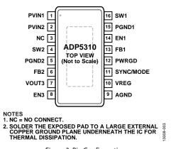
Figure 3. Pin Configuration
