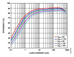
Figure 5. Channel 1 Auto PSM/PWM Efficiency vs. Load Current, V<sub>OUT1</sub> = 2.5 V
