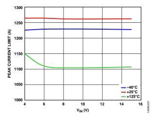
Figure 37. Channel 1 Peak Current Limit vs. V<sub>IN</sub>
