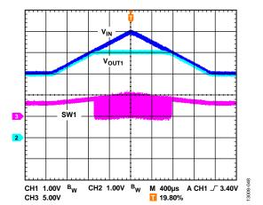
Figure 48. Channel 1 100% Duty Operation in PWM Mode
