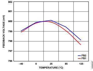
Figure 27. Channel 2 Feedback Voltage of PWM Mode vs. Temperature
