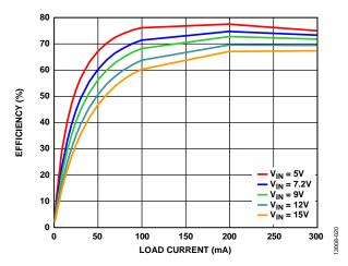
Figure 20. Channel 2 PWM Efficiency vs. Load Current,  $V_{OUT2} = 1.2 \text{ V}$
