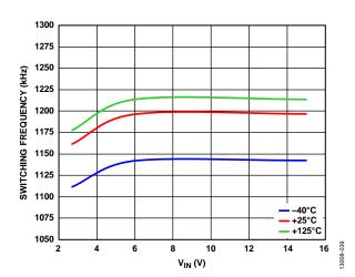
Figure 39. Switching Frequency vs. V<sub>IN</sub>
