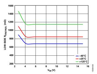
Figure 30. Channel 2 Low-Side R<sub>DS(ON)2L</sub> vs. V<sub>IN</sub>
