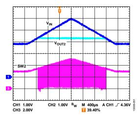
Figure 51. Channel 2 100% Duty Operation in PWM Mode
