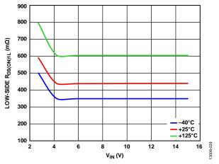
Figure 29. Channel 1 Low-Side RDS(ON)1L vs. VIN
