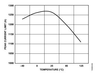
Figure 34. Channel 1 Peak Current Limit vs. Temperature
