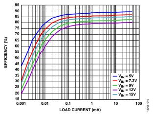
Figure 16. Channel 2 Hysteresis Efficiency vs. Load Current, V<sub>OUT2</sub> = 2.5 V
