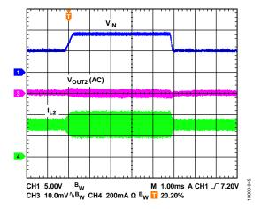
Figure 45. Channel 2 Line Transient in PWM Mode
