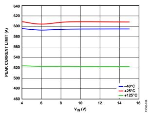
Figure 38. Channel 2 Peak Current Limit vs. V<sub>IN</sub>
