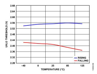
Figure 36. UVLO Threshold, Rising and Falling, vs. Temperature
