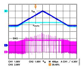
Figure 52. Channel 2 100% Duty Operation in Hysteresis Mode
