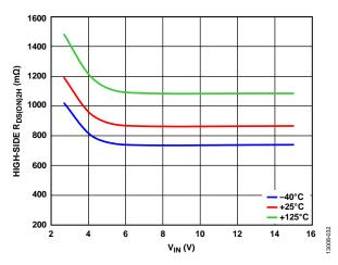
Figure 32. Channel 2 High-Side R<sub>DS(ON)2H</sub> vs. V<sub>IN</sub>
