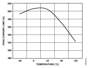
Figure 35. Channel 2 Peak Current Limit vs. Temperature
