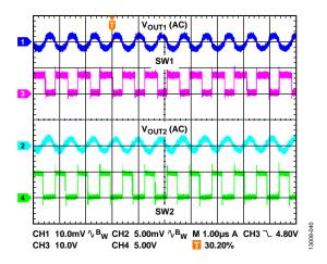
Figure 40. Steady Waveform of PWM Mode
