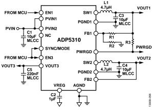
Figure 56. Typical Application Circuit
