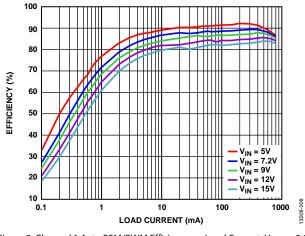
Figure 8. Channel 1 Auto PSM/PWM Efficiency vs. Load Current,  $V_{OUT1} = 3.3 \text{ V}$
