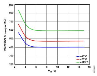
Figure 31. Channel 1 High-Side R<sub>DS(ON)1H</sub> vs. V<sub>IN</sub>
