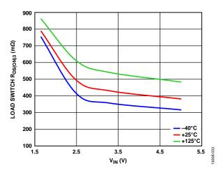
Figure 33. Channel 3 Load Switch  $R_{DS(ON)3}$  vs.  $V_{IN}$
