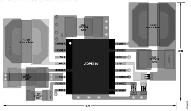
Figure 57. Typical PCB Layout for the ADP5310
