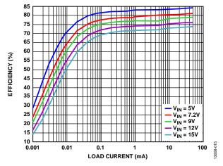
Figure 15. Channel 2 Hysteresis Efficiency vs. Load Current, V<sub>OUT2</sub> = 1.8 V
