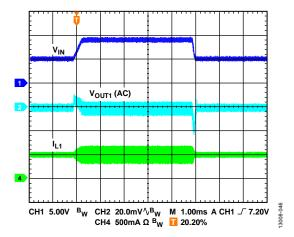
Figure 46. Channel 1 Line Transient in PWM Mode
