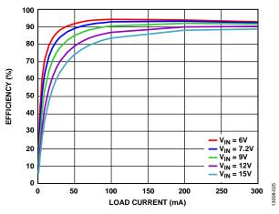
Figure 25. Channel 2 PWM Efficiency vs. Load Current,  $V_{OUT2} = 5 V$
