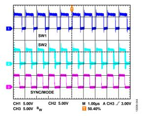
Figure 44. Synchronization to 1 MHz
