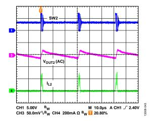
Figure 43. Channel 2 Output Ripple of Hysteresis Mode
