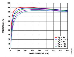
Figure 13. Channel 1 PWM Efficiency vs. Load Current,  $V_{OUT1} = 2.5 \text{ V}$
