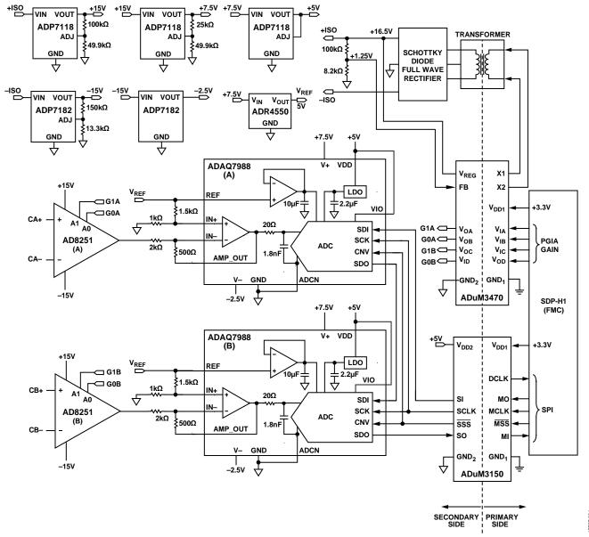
Figure 1. CN-0393 Simplified Schematic Diagram
