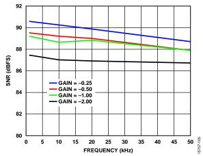
Figure 5. SNR vs. Input Frequency
