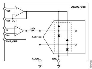
Figure 8. ADC Input ESD Diodes
