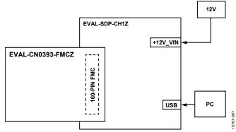
Figure 10. CN-0393 Evaluation Hardware Connections
