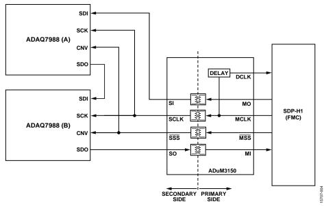
Figure 4. Digital Interface Simplified Schematic
