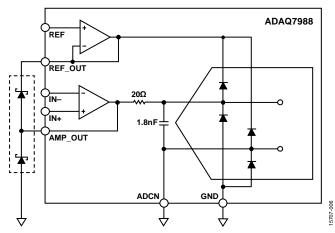
Figure 9. Using Schottky Diodes for Additional Overvoltage Protection
