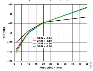
Figure 6. THD vs. Input Frequency
