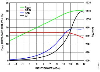
Figure 33. Pout, Gain, PAE, and IDD vs. Input Power, Frequency = 30 GHz
