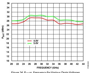
Figure 24. PSAT vs. Frequency for Various Drain Voltages
