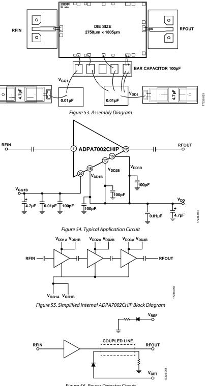
Figure 56. Power Detector Circuit
