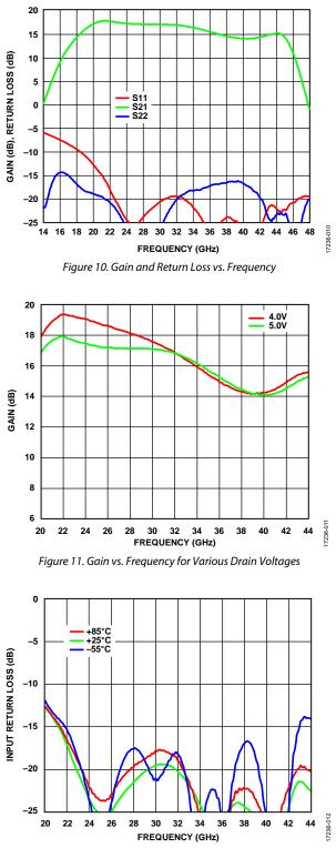
Figure 12. Input Return Loss vs. Frequency for Various Temperatures,  $V_{DD} = 5 V$ ,  $I_{DQ} = 600 \text{ mA}$
