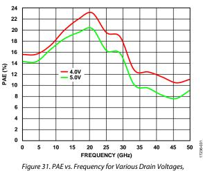
igure 31. PAE vs. Frequency for Various Drain Voltage: PAE Measured at P<sub>saτ</sub>
