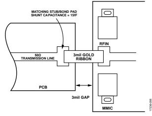
Figure 67. High Frequency Input Wideband Matching
