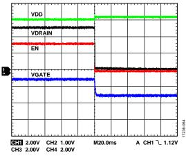
Figure 62. Turn Off—HMC980LP4E Outputs to the ADPA7002CHIP
