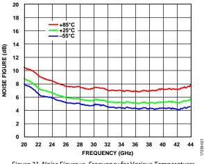
Figure 21. Noise Figure vs. Frequency for Various Temperatures
