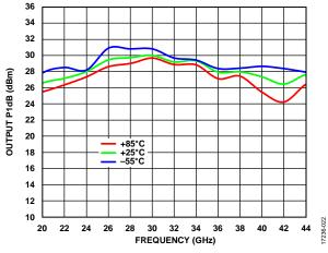
Figure 22. Output P1dB vs. Frequency for Various Temperatures
