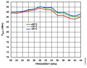
Figure 49. P<sub>SAT</sub> vs. Frequency for Various Temperatures, Data Measured with Constant I<sub>DD</sub>
