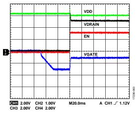
Figure 61. Turn On—HMC980LP4E Outputs to the ADPA7002CHIP
