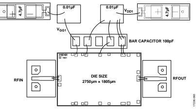
Figure 57. Alternate Assembly Diagram
