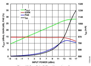
Figure 37. POUT, Gain, PAE, and IDD vs. Input Power, Frequency = 38 GHz
