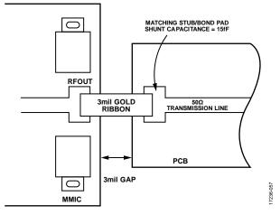
Figure 68. High Frequency Output Wideband Matching
