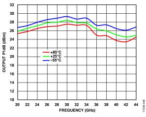
Figure 48. Output P1dB vs. Frequency for Various Temperatures, Data Measured with Constant I<sub>DD</sub>
