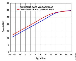
Figure 64.  $P_{OUT}$  vs.  $P_{IN}$  for Constant Gate Voltage Bias and Constant Drain Current Bias,  $V_{DD} = 5 V$ , Frequency = 32 GHz
