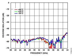
Figure 18. Reverse Isolation vs. Frequency for Various Temperatures
