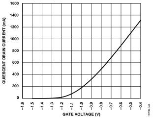
Figure 46. Quiescent Drain Current vs. Gate Voltage
