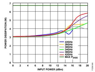
Figure 38. Power Dissipation vs. Input Power,  $T_A = 85^{\circ}C$
