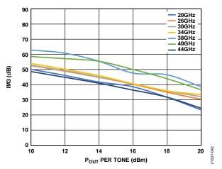
Figure 41. IM3 vs.  $P_{OUT}$  per Tone at Various Frequencies,  $V_{DD} = 4 V$ ,  $I_{DQ} = 800 \text{ mA}$
