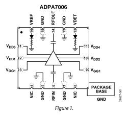
countermeasure and instrumentation applications requiring >27 dBm of efficient saturated output power. The RF inputs and outputs are internally matched and dc blocked for ease of integration into higher level assemblies. The ADPA7006 is housed in a 6 mm  $\times$  6 mm, 16-terminal ceramic leadless chip carrier with heat sink (LCC\_HS) that exhibits low thermal resistance and is compatible with surface-mount manufacturing techniques.
