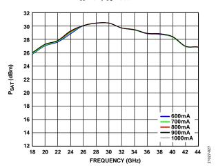
Figure 27.  $P_{SAT}$  vs. Frequency for Various  $I_{DQ}$ ,  $V_{DD} = 5 \text{ V}$
