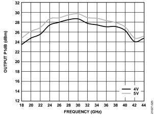
Figure 25. Output P1dB vs. Frequency for Various  $V_{DD}$ ,  $I_{DQ} = 800 \text{ mA}$
