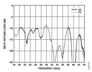
Figure 15. Input Return Loss vs. Frequency for Various  $V_{DD}$ ,  $I_{DQ} = 800 \text{ mA}$
