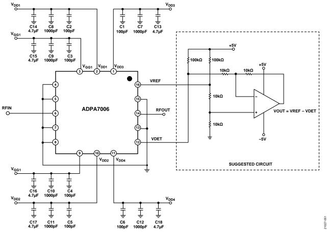
Figure 52. Typical Application Circuit
