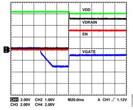
Figure 57. Turn On HMC980LP4E Outputs to the ADPA7006
