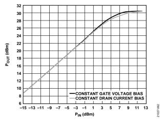
Figure 60.  $P_{OUT}$  vs.  $P_{IN}$ ,  $V_{DD} = 5$  V, Frequency = 32 GHz, Constant Drain Current Bias ( $I_{DRAIN}$  Setpoint = 1000 mA) and Constant Gate Voltage Bias ( $V_{GGI} \approx -0.68$  V)
