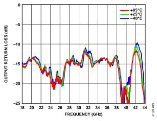
Figure 19. Output Return Loss vs. Frequency for Various Temperatures,  $V_{DD} = 5 \text{ V}$ ,  $I_{DQ} = 800 \text{ mA}$
