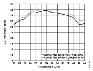
Figure 62. Output P1dB vs. Frequency,  $V_{DD} = 5$  V, Constant Drain Current Bias ( $I_{DRAIN}$  Setpoint = 1000 mA) and Constant Gate Voltage Bias ( $V_{GGI} \approx -0.68$  V)
