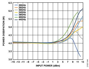
Figure 43. Power Dissipation vs. Input Power at Various Frequencies,  $T = 85^{\circ}\text{C}$ ,  $V_{DD} = 5 \text{ V}$ ,  $I_{DQ} = 800 \text{ mA}$
