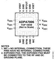
Figure 2. Pin Configuration
