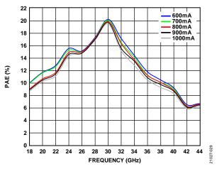
Figure 29. PAE vs. Frequency for Various  $I_{DQ}$ ,  $V_{DD} = 5 V$ , PAE Measured at  $P_{SAT}$
