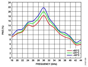
Figure 28. Power Added Efficiency (PAE) vs. Frequency for Various Temperatures,  $V_{DD} = 5 V$ ,  $I_{DQ} = 800 \text{ mA}$ , PAE Measured at  $P_{SAT}$
