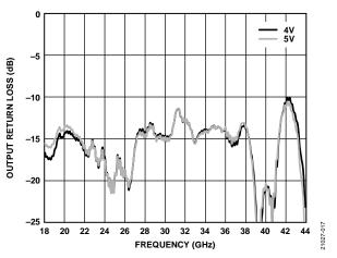
Figure 17. Output Return Loss vs. Frequency for Various  $V_{DD_{r}}$  $I_{DQ} = 800 \text{ mA}$
