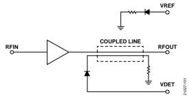
Figure 51. Power Detector Circuit
