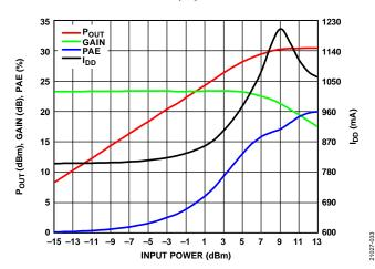
Figure 33.  $P_{OUT}$ , Gain, PAE, and  $I_{DD}$  vs. Input Power, 30 GHz,  $V_{DD} = 5 V$ ,  $I_{DQ} = 800 \text{ mA}$
