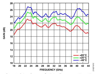
Figure 13. Gain vs. Frequency for Various Temperatures,  $V_{DD} = 5 V$ ,  $I_{DQ} = 800 \text{ mA}$
