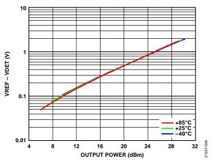
Figure 45. Detector Voltage (VREF - VDET) vs. Output Power for Various Temperatures at 32 GHz,  $V_{DD} = 5 V$ ,  $I_{DQ} = 800 \text{ mA}$
