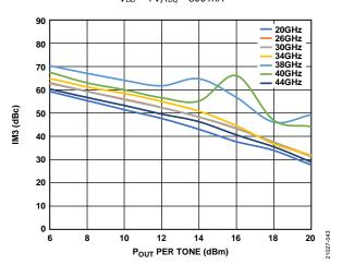
Figure 42. Third-Order Intermodulation Distortion Relative to Carrier (IM3) vs.  $P_{OUT}$  per Tone at Various Frequencies,  $V_{DD} = 5 V$ ,  $I_{DQ} = 800 \text{ mA}$
