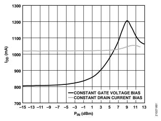
Figure 59.  $I_{DD}$  vs.  $P_{IN}$ ,  $V_{DD}$  = 5 V, Frequency = 30 GHz, Constant Drain Current Bias ( $I_{DRAIN}$  Setpoint = 1000 mA) and Constant Gate Voltage Bias ( $V_{GGI} \approx -0.68 \text{ V}$ )
