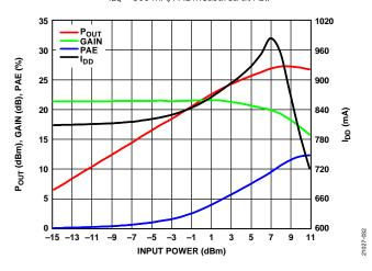
Figure 32.  $P_{OUT}$ , Gain, PAE, and  $I_{DD}$  vs. Input Power, 20 GHz,  $V_{DD} = 5 \text{ V}$ ,  $I_{DQ} = 800 \text{ mA}$
