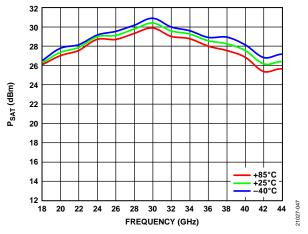
Figure 47.  $P_{SAT}$  vs. Frequency for Various Temperatures,  $V_{DD} = 5 V$ ,
