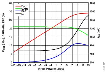
Figure 36.  $P_{OUT}$ , Gain, PAE, and  $I_{DD}$  vs. Input Power, 38 GHz,  $V_{DD} = 5 V$ ,  $I_{DQ} = 800 \text{ mA}$
