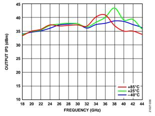
Figure 37. Output IP3 vs. Frequency for Various Temperatures,  $P_{OUT}$  per Tone = 16 dBm,  $V_{DD}$  = 5 V,  $I_{DQ}$  = 800 mA
