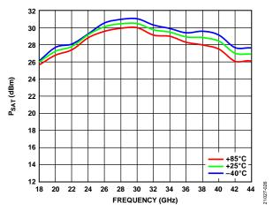
Figure 26.  $P_{SAT}$  vs. Frequency for Various Temperatures,  $V_{DD} = 5 V$ ,  $I_{DQ} = 800 \text{ mA}$
