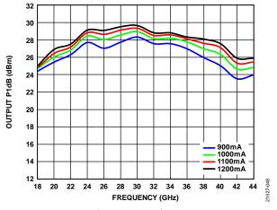
Figure 48. Output P1dB vs. Frequency for Various Drain Currents,  $V_{DD} = 5 V$ , Data Measured with Constant  $I_{DD}$
