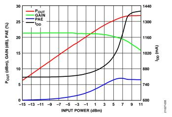
Figure 34.  $P_{OUT}$ , Gain, PAE, and  $I_{DD}$  vs. Input Power, 44 GHz,  $V_{DD} = 5 V$ ,  $I_{DQ} = 800 \text{ mA}$
