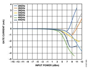
Figure 44. Gate Current vs. Input Power at Various Frequencies,  $V_{DD} = 5 V$ ,  $I_{DQ} = 800 \text{ mA}$
