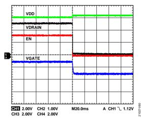
Figure 58. Turn Off HMC980LP4E Outputs to the ADPA7006
