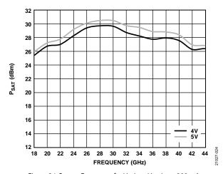
Figure 24.  $P_{SAT}$  vs. Frequency for Various  $V_{DD}$ ,  $I_{DQ} = 800 \text{ mA}$
