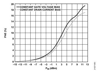
Figure 61. PAE vs. Input Power,  $V_{DD} = 5$  V, Frequency = 30 GHz, Constant Drain Current Bias ( $I_{DRAIN}$  Setpoint = 1000 mA) and Constant Gate Voltage Bias ( $V_{GGI} \approx -0.68$  V)
