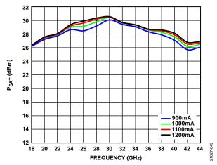
Figure 49.  $P_{SAT}$  vs. Frequency for Various Drain Currents,  $V_{DD} = 5 V$ ,
