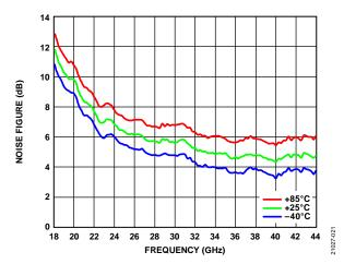
Figure 21. Noise Figure vs. Frequency for Various Temperatures,  $V_{DD} = 5 V$ ,  $I_{DQ} = 800 \text{ mA}$
