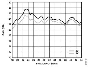
Figure 11. Gain vs. Frequency for Various  $V_{DD}$ ,  $I_{DQ} = 800 \text{ mA}$
