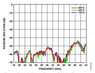
Figure 18. Reverse Isolation vs. Frequency for Various Temperatures,  $V_{DD} = 5 V$ ,  $I_{DQ} = 800 \text{ mA}$
