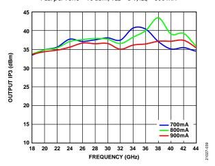
Figure 38. Output IP3 vs. Frequency for Various  $I_{DQ}$ ,  $P_{OUT}$  per Tone = 16 dBm,  $V_{DD}$  = 5 V
