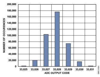
Figure 4. Histogram of a DC Input at the Code Center for 390,000 Samples
