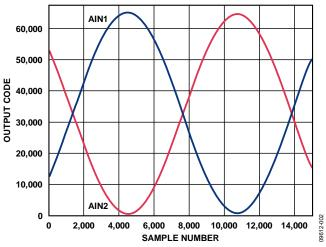
Figure 2. 15,000 Samples of Two Separate ±10V Input Signals (AIN1,AIN2), 90° Out of Phase, Applied to AIN1 and AIN2 Sampled at 250 kSPS on the EVAL-CN0194-SDPZ Board in Daisy Chain Mode
